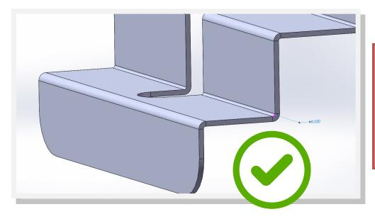
**NOTE:** RAPID recommends keeping the same bend radii across all bends when possible. This helps minimize the amount of brake setups and keeps cost down.
