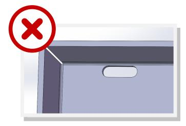
**NOTE:** If using eRAPID, all holes and cutouts need to be a minimum of 4x the material thickness away from the material edge to avoid additional costs in estimating.
