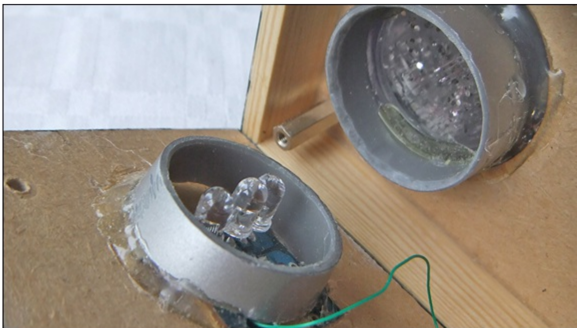
Figure 12-7: The lamp/electronics assembly.
