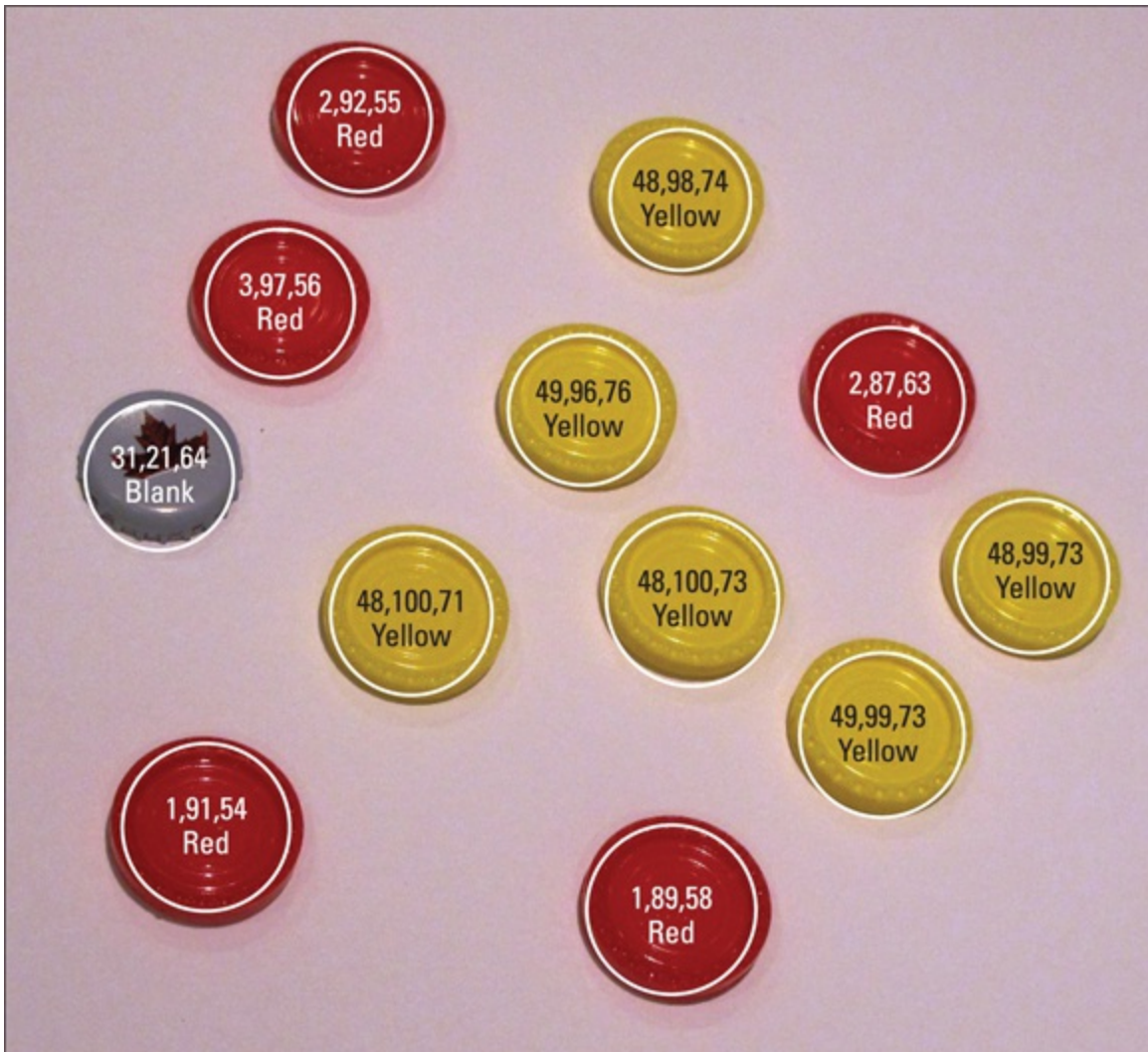
Figure 11-4: Circle and color detection with OpenCV.
