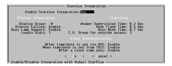
The Vodavi Integration window is located under the System Options menu button. See KI-2000 TCKS1401 Telecenter<sup>®</sup> / STARPLUS<sup>®</sup> Integration for details on integrating the TC21 with the Vodavi STARPLUS. (*The Vodavi Starplus Integration feature is available in firmware version 3.0 and later.*)
