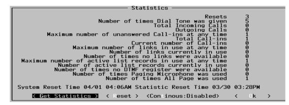
The *Statistics* dialog shows how heavily the system has been used. For example, it will list call-ins, incoming and outgoing calls, pages (both from telephones and from the Priority Microphone), and how many times all the DTMF registers were tied up. It also shows the time and date when the system was last reset and when the statistics file was reset. If system power is lost, both the system and the *Statistics* file will reset and the time and date will be recorded.
