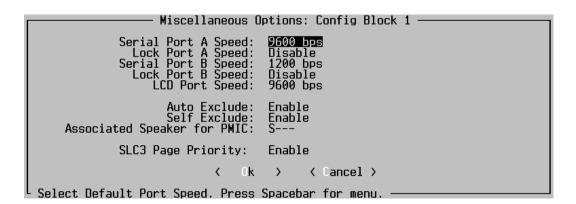
This menu controls the baud rates of the system ports and some speaker-exclude functions. Port A settings take effect on reset or power-up; Port B settings take effect immediately after program changes have been sent down via F9.
