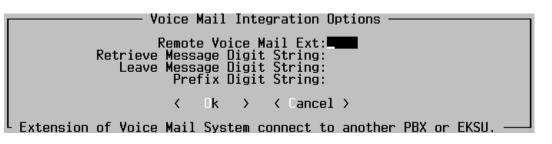
This screen configures the various dialing strings sent to a voice mail system when a call is forwarded to or when the voice mail system is called directly. See Appendix F for details on how to integrate the Telecenter System 21 with a local (directly connected) or remotely (attached to another PBX or EKSU) voice mail system. .(*The Voice Mail Integration Feature is avaiable in firmware version 4.0 and later.*)
