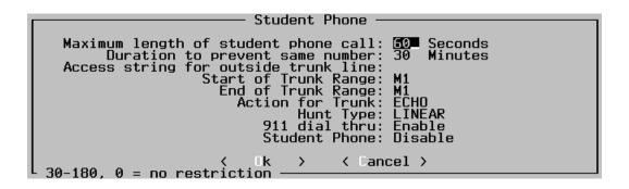
These settings control most of the functions of Student Phone<sup>™</sup> lines. The Class-of-Service settings (in the "Communications" section) control access for local and toll calls.
