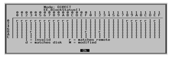
Select this file to see how the copy of the user programming that you are working on (the workspace copy) compares with an open file or the stored programming information from the TC2100 system.
