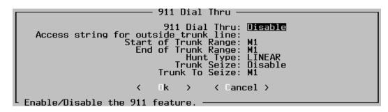
When this feature is activated, any dialing phone in the system can dial the regular "911" emergency number and have the call forwarded to a central-office line.
