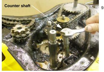
Double nut the counter shaft and remove the nut, lock washer and Belleville washer from the bottom of the shaft using an 11/16" wrench. See Figure 5.68.
