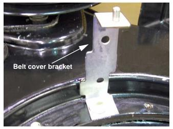
13. Remove the hex nut and lock washer from the mounting stud on the belt cover bracket using a 1/2" wrench, and remove the bracket. See Figure 5.16.
