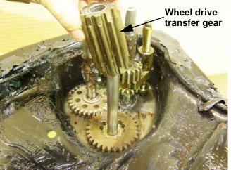
7. Below the main shaft wheel gear is a wheel drive transfer gear. Lift it off of the main shaft. See Figure 5.42.
