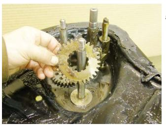
8. Lift the bottom (reverse wheel drive) gear off of the main shaft. See Figure 5.43.
