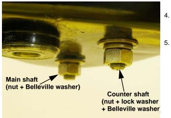
Remove the nut, lock washer, and Belleville washer from the bottom of the counter shaft using an 11/16" wrench. See Figure 5.47.
