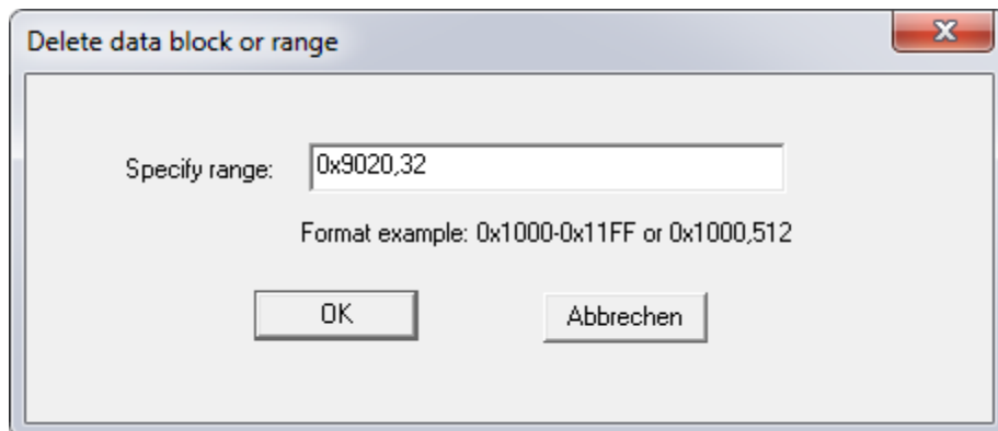
Figure 2-20 Example of cut-data using start-address and length as a parameter
