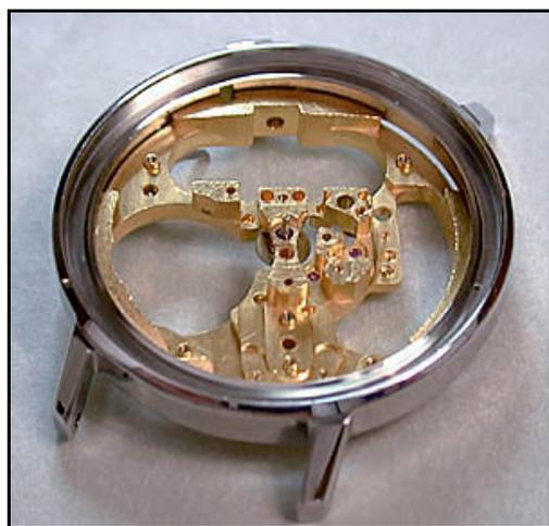
On first examination, one of the most startling aspects of the Accutron is how much traditional, high grade watchmaking is involved in its design and execution. It uses an extremely well-made, traditional, machined brass ebauche (**left**) with a highly jeweled gear train. Most of the gear train uses conical pivots with pierced and cap jewels, and nearly half the gear train is shock protected.
