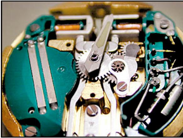
standard derived from the minuscule vibrations of a tuning fork actually translate into both timing and powering the hands of a watch?
