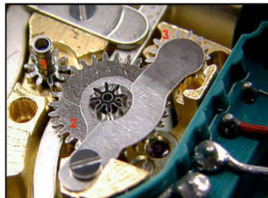
The gear train of the Accutron resembles that of a high-grade mechanical movement (**right**). We might even imagine that we were observing a center wheel (1), third wheel (2), fourth wheel (3), escape wheel (4), and . . . well, it's not a balance wheel, it's the *drive wheel* (5). More about that drive wheel in a moment.
