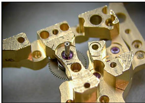
On the dial side of the movement (**right**) we find a conventional cannon pinion (1) to carry the minute hand, as well as a minute wheel (2) to drive the hour hand. Even the hand-setting mechanism employs an intermediate wheel (3) that could be lifted from the most traditional of mechanical movements.
