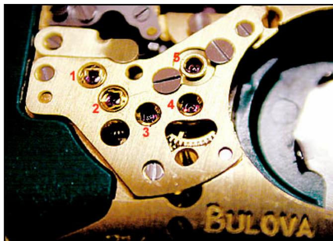
With the wheel train bridge in place, we see the remarkable jeweling of the movement. The drive wheel (1) and (now in Accutron parlance) second wheel (2) each use four jewels and shock protection top and bottom. The third, fourth, and center wheels (3, 4, and 5) are fully jeweled with cylindrical pivots. Note the chaton for the center wheel (5). This is a high-precision, low drag gear train.
