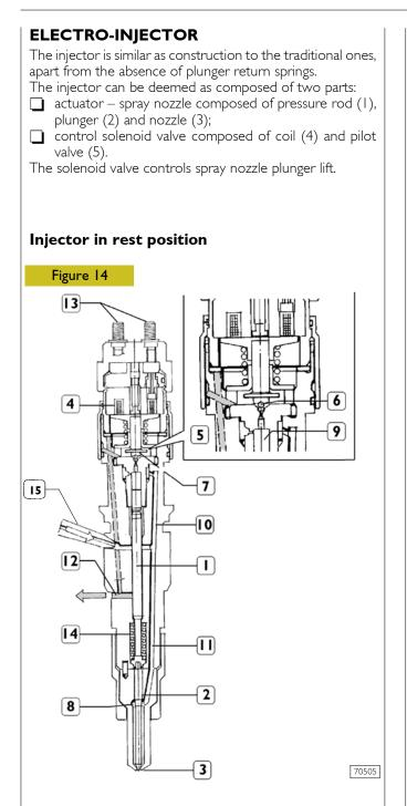
Pressure rod – 2. Plunger – 3. Nozzle – 4. Coil – 5. Pilot valve – 6. Ball shutter – 7. Control area – 8. Pressure chamber – 9. Control volume – 10. Control duct – 11. Supply duct – 12. Control fuel outlet – 13. Electric connection – 14. Spring – 15. High-pressure fuel inlet.
