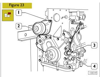
Remove the screws (1) and disconnect the water pump (2). Remove the screw (3) and the roller (4).
