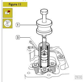
Remove injector fastening screws. Use tool 99342101 (1) to remove injectors (2) from the cylinder head.
