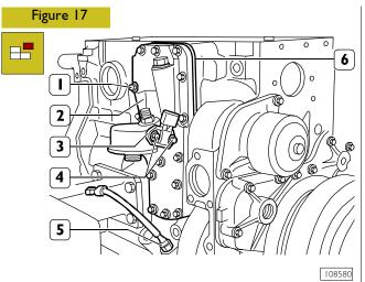
Remove the screws (4) and disconnect the oil temperature/pressure sensor (3).
