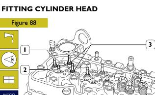
Lubricate the valve stems (1) and fit them into the relevant valve guides according to the position marked at removal.
