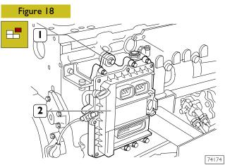
Remove the screws (1) and disconnect the ECU (2) including the heat exchanger.
