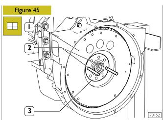
Screw two pins (2) having suitable length into shaft holes (3) and remove the engine flywheel (1) using proper sling and hoister.
