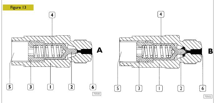
I. Body – 2. Small piston – 3. Stop – 4. Spring – 5. Direct tank discharge – 6. Seat on rail.
