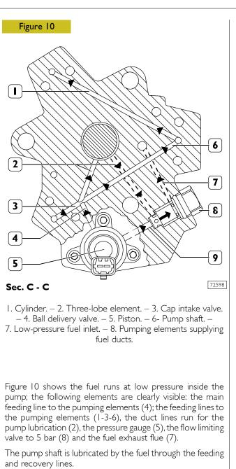
The pressure gauge (5) determines the quantity of fuel to feed the pumping elements: the fuel in excess flows through the exhaust gallery (9).
