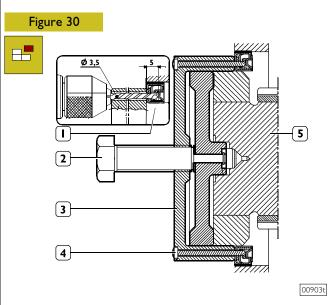
Remove the holding ring of the flywheel cover box using the tool 99340056 (3) to operate on the driving shaft's back bar hold (5).
