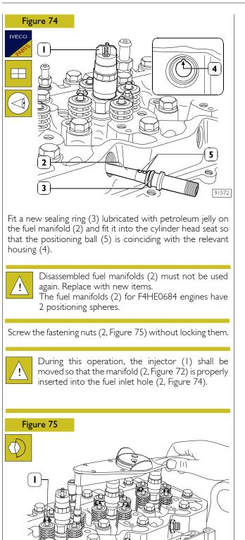
Use the torque wrench to tighten gradually and alternately the injector fastening screws (1) to  $8.5 \pm 0.8$  Nm torque.
