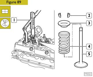
Position on the cylinder head: the spring (4), the upper cap (3); use tool 99360268 (1) to compress the spring (4) and lock the parts to the valve (5) by the cotters (2).
