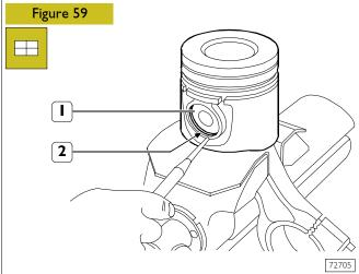
Position the piston (1) on the connecting rod according to the diagram shown in the figure, fit the pin (3) and stop it by the split rings (2).
