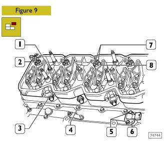
Remove nuts (7) and disconnect the electrical cables from injectors (8).
