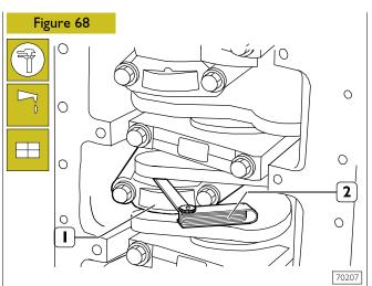
If a different clearance value is found, replace the half bearings and repeat the check.
