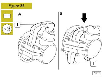
Press the clamp (1) in arrow direction (Figure B) and connect the pipe to the rail, reset the clamp to the initial locking position "A".
