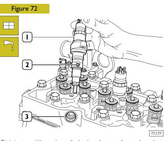
Fit injectors (1) on the cylinder head seats, directed so that the fuel inlet hole (2) is facing the fuel manifold seat (3) side.
