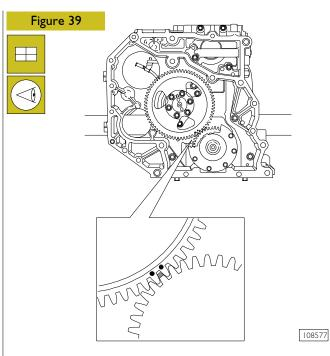
Rotate the output shaft (4) and the camshaft (2) so that when fitting the driven gear (1) on the camshaft the marks on the gears (1 and 3) are coinciding.
