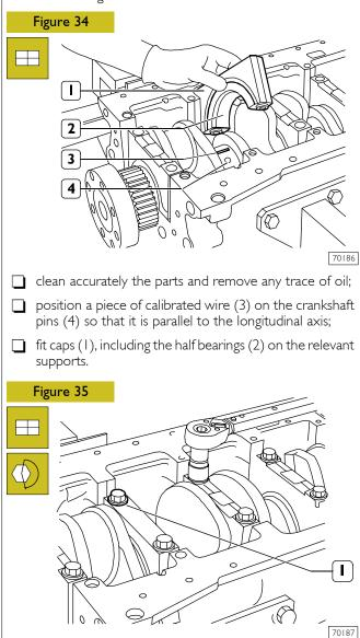
Tighten the pre-lubricated screws (1) in the following three successive stages:
