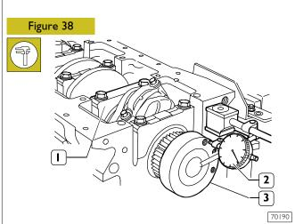
This check is performed by setting a magnetic-base dial gauge (2) on the crankshaft (3) as shown in the figure, standard value is 0.068 to 0.41.
