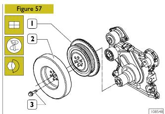
Assemble the pulley (1) and the damping flywheel (2) to the driving shaft.
