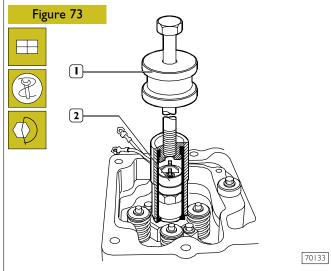
Use tool 99342101 (1) to fit the injector (2) into its seat. Screw injector fastening screws without tightening them.
