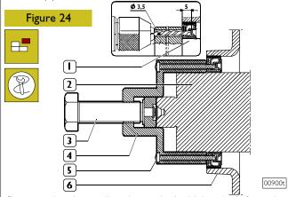
Remove the ring sealing the engine's driving shaft from the front cover. Use the tool 99340055 (4) to operate on the front bar hold of the driving shaft. Through the steering holes of the tool, perforate the inside holding ring (1) with a straight way drill (diam. 3,5mm) for the depth of 5mm. Fix the tool to the ring tightening the 6 screws provided with the equipment. Then proceed removing the ring (2) by tightening the screw (3).
