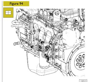
Assemble the bracket and the support (1) of the fuel filter (6). Proceed connecting in sequence the pipelines (9,3,4 and 5) of the support (1) to the high pressure pump (8).
