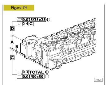
The rated thickness A for the cylinder head is  $105 \pm 0.25$  mm, max. metal removal shall not exceed thickness B by 1 mm.
