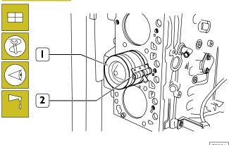
Lubricate accurately the pistons, including the split rings and the cylinder barrel inside.
