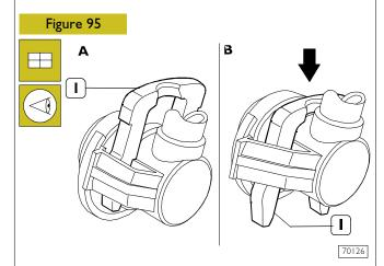
All the fuel pipelines are fixed using the clamps shown in the picture.
