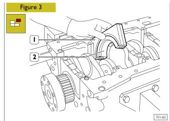
The second last main bearing cap (1) and the relevant support are fitted with shoulder half-bearing (2).
