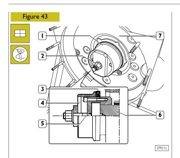
Apply tool 99346252 part (6) to the rear output shaft tang (5), secure it by screws (4) and fit the new sealing ring (3). Position part (1) on part (5), screw nut (2) until completing sealing ring (3) fitting into flywheel housing (7).
