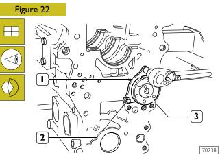
Set camshaft (3) retaining plate (1) with the slot facing the top of the engine block and the marking facing the operator, then tighten the screws (2) to the specified torque.
