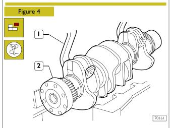
Use tool 99360500 (1) and hoist to remove the crankshaft (2) from the block.
