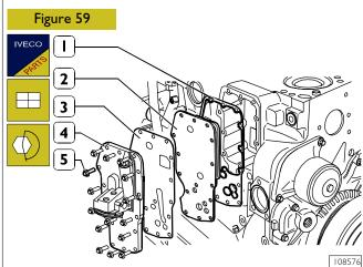
Fit on the engine block: a new gasket (1), the heat exchanger (2) a new gasket (3) and the oil filter support (4).
