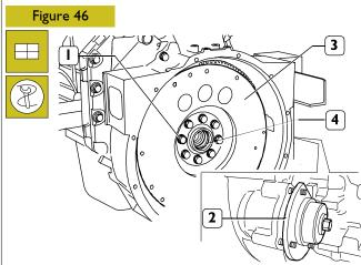
Apply tool 99360339 (2) to the flywheel housing to stop engine flywheel (3) rotation. Tighten the screws (1) fastening the engine flywheel (3) to the output shaft.
