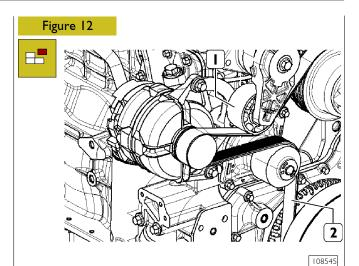
Release on the drive belt tensioner (1) and extract the belt (2) from the belt pulleys from the water pump ones and from the belt rebound pulleys;
