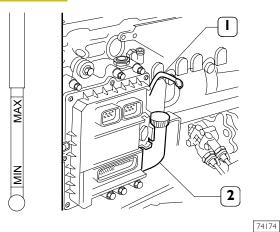
Draw off the rod from its slot and check that the level is within the etched tags of minimum and maximum level.
