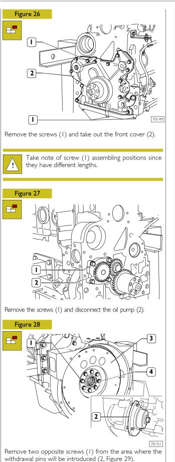
Loosen the remaining flywheel fixing screws (3) from the driving shaft (4).
