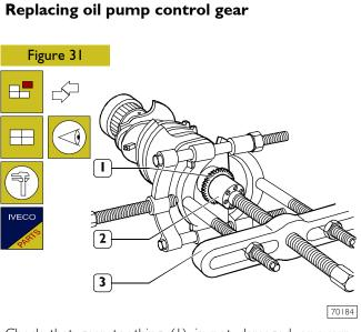
Check that gear toothing (1) is not damaged or worn, otherwise remove it using the proper puller (3).
