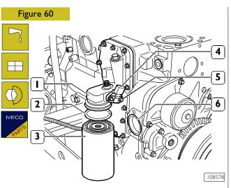
Lubricate the sealing ring (2) with engine oil and set it on the oil filter (3).
