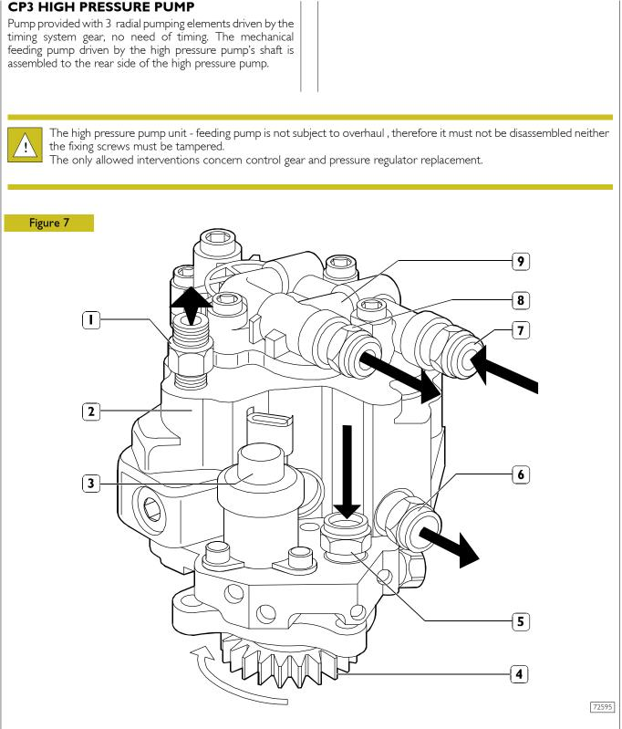
I. Fuel exhaust connector to rail - 2. High pressure pump - 3. Pressure regulating gauge - 4. Driving gear - 5. Connector to fuel entry flowing from filter - 6. Connector to fuel exhaust to filter support - 7. Connector to fuel entry flowing from engine control module heat exchanger - 8. Connector to fuel exhaust flowing from mechanic pump to filter - 9. Mechanical feeding pump.
