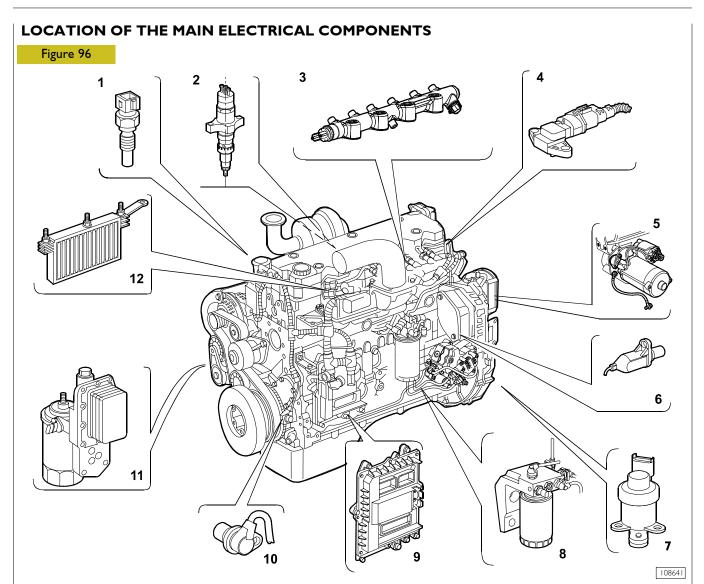
The NEF F4HE engines are fully driven by the electronic engine control module, which is assembled directly to the engine by means of a heat exchanger enabling its cooling, utilising rubber buffers to reduce vibration originated by the engine.
