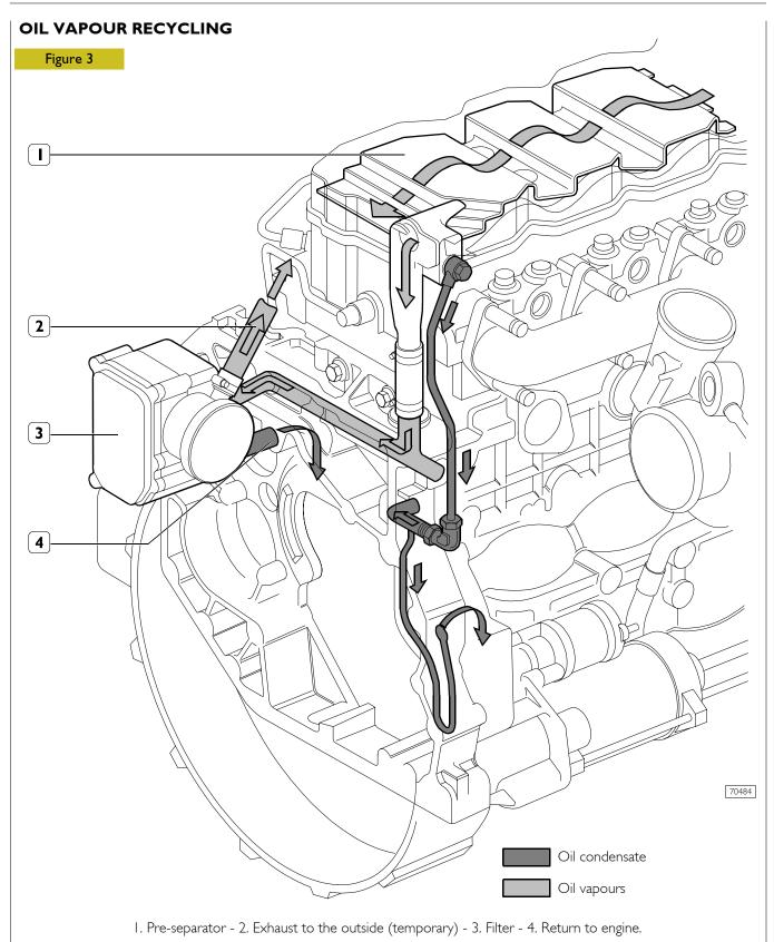
The tappet cover houses the pre-separator (1), whose shape and position determines an increase in oil vapour outlet speed and condenses a part of vapours at the same time.
