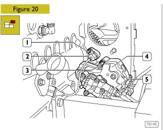
Remove the nut (1) and disconnect the timing sensor (2).
