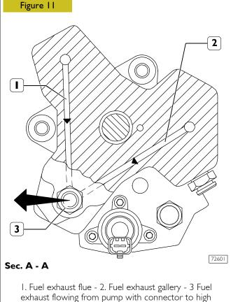
Figure 11 shows the fuel flow under high pressure running through the exhaust galleries of the pumping elements.
