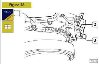
Fit a new sealing ring on the speed sensor (3).
