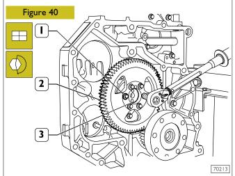
Tighten the screws (1) fastening gear (2) to camshaft (3) to the specified torque.
