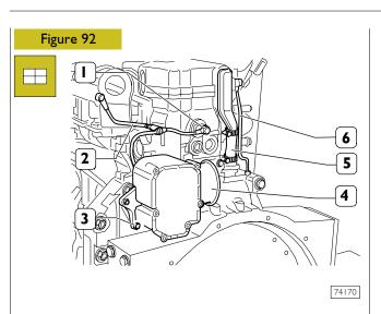
Insert the blow-by filter (4) tightening the screws.
