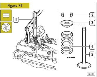
Valve removal shall be performed using tool 99360268 (1) and pressing the cap (3) so that when compressing the springs (4) the cotters (2) can be removed. Then remove the cap (3) and the springs (4).
