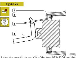
Using the specific tie rod (3) of the tool 99363204 and the ancillary lever (4), remove the external holding ring (2) from the front cover (1).
