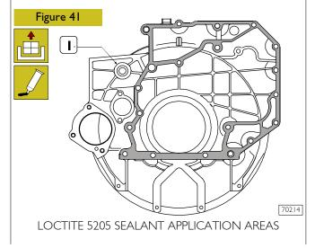
Perfect seal is only obtained by cleaning accurately the surface to seal.
