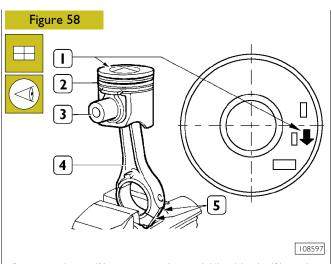
Connect piston (2) to connecting rod (4) with pin (3) so that the reference arrow (1) for fitting the piston (2) into the cylinder barrel and the numbers (5) marked on the connecting rod (5) are read as shown in the figure.
