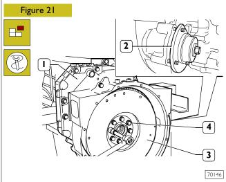
Fit tool 99360339 (2) to the flywheel housing (1) to stop flywheel (3) rotation.
