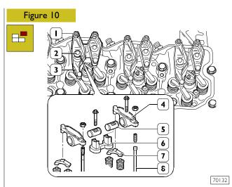
Loosen tappet adjustment fastening nuts (  ${\sf I}$  ) and unscrew the adjusters.
