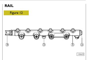
Rail – 2. Fuel inlet from high-pressure pump –
