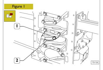
Loosen the fixing screws (1) and remove the rod caps (2). Withdraw the pistons including the connecting rods from the top of the engine block.
