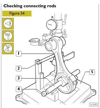
Check that the axis of the connecting rods (1) are parallel using tool 99395363 (5) as follows:
