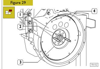
Tighten two screws of medium length into the holes (4) to sling the flywheel with the hoist.
