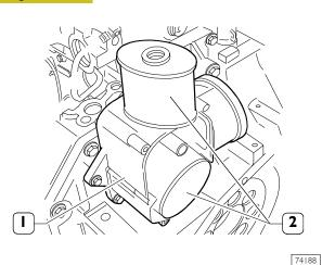
The check of the filtering element is carried out by removing the cover and drawing off the cartridges (2).
