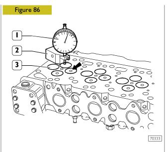
After regrinding, check that value (3) sinking value is the specified one by using the base 99370415 (2) and the dial gauge 99395603 (1).
