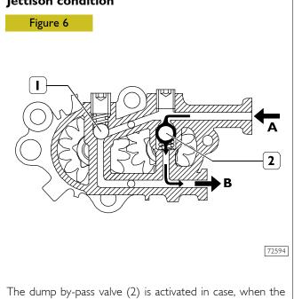
Ine dump by-pass valve (2) is activated in case, when the engine is off, it is necessary to fill the feeding system through the priming pump. In this condition the by pass valve (1) keeps closed while the dump by-pass valve (2) opens up due to the pressure effect on the entry unit so the fuel flows to the exhaust unit B.
