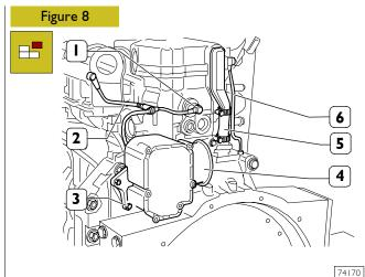
Disconnect the pipeline (2) from the fuel recover pressure-limiter, working on the connections as described in Figure 3.
