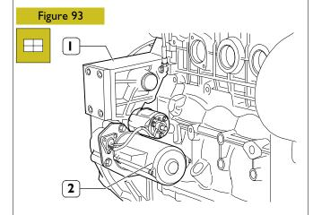
Assemble the starter (2) to the internal part of the flywheel cover.
