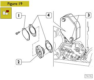
Unloose the screws (3) and remove the cap (1). Keep the gasket (4), the power take-off (2) and the second gasket (4).
