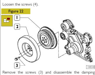
Remove the screws (3) and disassemble the damping flywheel (2) and the pulley (1).
