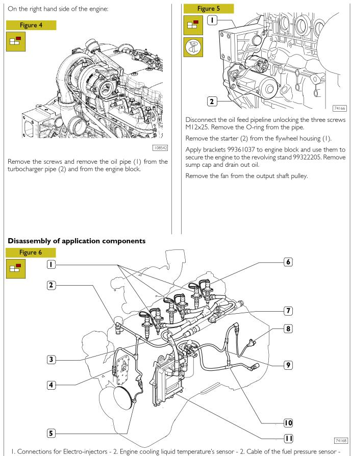
Connections for Electro-injectors - 2. Engine cooling liquid temperature's sensor - 2. Cable of the fuel pressure sensor -4. Sensor of engine's oil temperature and pressure - 5. Driving shaft sensor - 6. Electro-injector - 7. Temperature - air pressure sensor - 8. Timing system sensor - 9. Cable of fuel heater and fuel temperature's sensor - 10. Cable of pressure regulating gauge - 11. EDC 7 gearbox.
