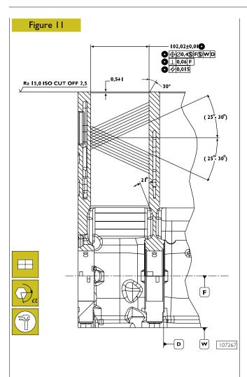
In case of regrinding, all barrels shall have the same oversize (0.5 mm).
