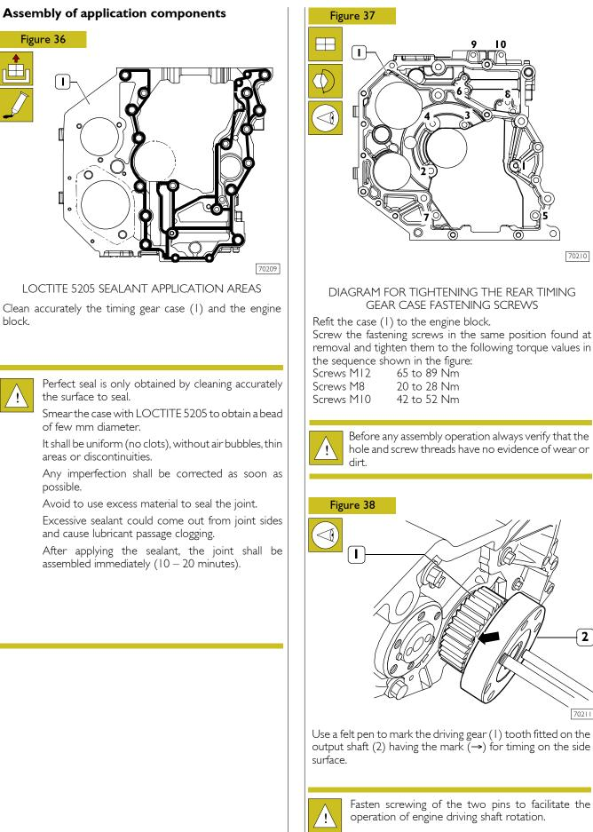
Fasten screwing of the two pins to facilitate the operation of engine driving shaft rotation.
