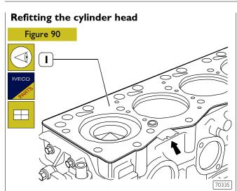
Check cleanness of cylinder head and engine block coupling surface.
