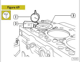
Once connecting rod-piston assemblies refitting is over, use dial gauge 39395603 (1) fitted with base 99370415 (2) to check piston (3) protrusion at T.D.C. with respect to the top of the engine block.
