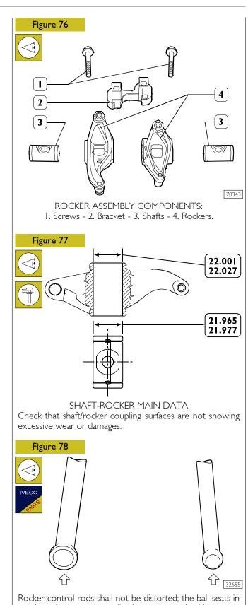
Rocker control rods shall not be distorted; the ball seats in touch with the rocker adjusting screw and with tappets (arrows) shall not show seizing or wear; otherwise replace them. Intake and exhaust valve control rods are identical and are therefore interchangeable.
