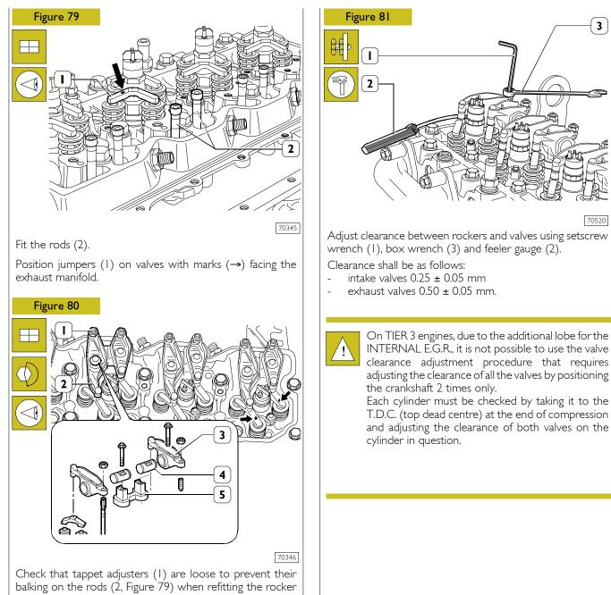
assembly. Then refit the rocker assembly consisting of: bracket (5), rockers (3), shafts (4) and secure them to the cylinder head
