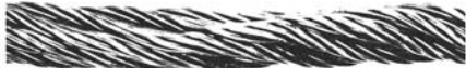
CRUSHING. Because of loose winding on drum, rope was pulled inbetween underlying wraps and crushed out of shape.
