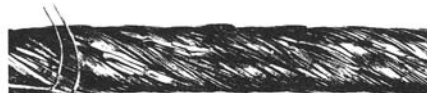
INFREQUENT INSPECTION. Neglect of periodical inspection left this rope in service too long, resulting in considerable abrasion.
