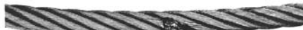
POOR WORK PROCEDURES. Damage to strands and wires resulted from electric arcing.
