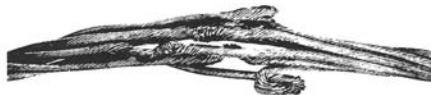
LACK OF KNOWLEDGE. Here's what occurs when a loop which has been "pulled through" and tightened remains in service.
