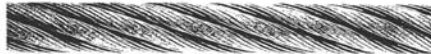
EXCESSIVE EXPOSURE TO ELEMENTS. Too much exposure combined with surface wear and loss of lubrication caused corrosion and pitting.
