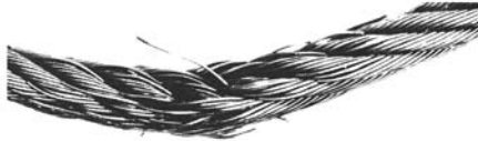
REVERSE BENDING Running this rope over one sheave and under another caused fatigue breaks in wires.
