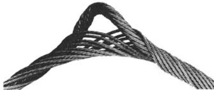
TOO SUDDEN LOAD RELEASE. The sudden release of a load caused birdcaging. Here individual strands open away from each other, displacing the core.
