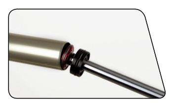
Push the rebound seal head firmly into the upper tube until the retaining ring groove is visible.
