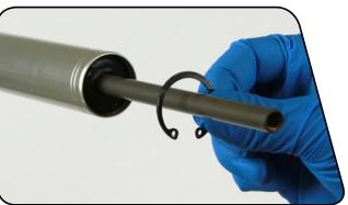
Firmly pull on the air shaft to remove the air shaft assembly from the upper tube. Clean and inspect the assembly for damage.
