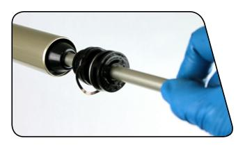
**Z** Spray isopropyl alcohol on the inside and outside of the upper tube. Wipe the outside of the upper tube with a clean rag.
