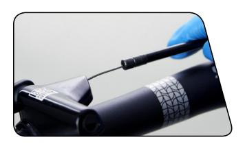
Use a 2 mm hex wrench to open the cable hatch cover.
