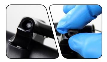
**RLT:** Wrap the cable around the spool and insert it through the cable fixing port. While firmly pulling the cable, use a 2 mm hex wrench to tighten the cable pinch bolt to 0.9 N·m (8 in-lb).
