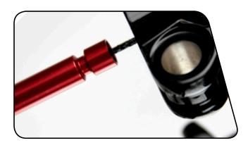
Refer to the air chart on the fork lower leg and pressurize the air spring to the appropriate pressure for your rider weight.
