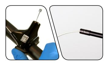
Pull the cable until the cable head is seated in the remote lever. With the cable head seated in the remote lever, close the cable hatch cover and push the lever to return it to the unlocked position.
