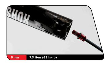
8 Insert the external rebound damper knob into the rebound damper shaft bolt until it is secure. Adjust the rebound.
