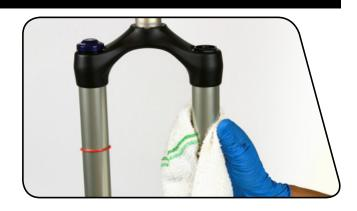
Apply a liberal amount of Buzzy's\* Slick Honey grease to the inner surfaces of the dust wiper seals.
