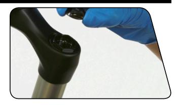
Use a small hex wrench to depress the Schrader valve and release all of the air pressure from the air chamber.
