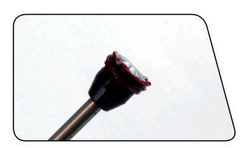
Apply a liberal amount of grease 40-60 mm around the air shaft. Install the floating seal head, a new floating seal head topout bumper, new aluminum support washer, new wavy washer and the air shaft guide, in that order, onto the air shaft.
