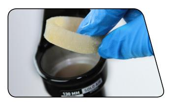
Soak the new foam rings in RockShox 15wt suspension fluid. Reinstall new foam rings on the top bushings in the lower legs.
