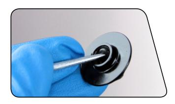
Place the tips of large internal snap ring pliers into eyelets of the snap ring, located at the bottom of the non-drive side upper tube. Press firmly on the pliers to push the air shaft guide into the upper tube enough to compress and remove the snap ring.
