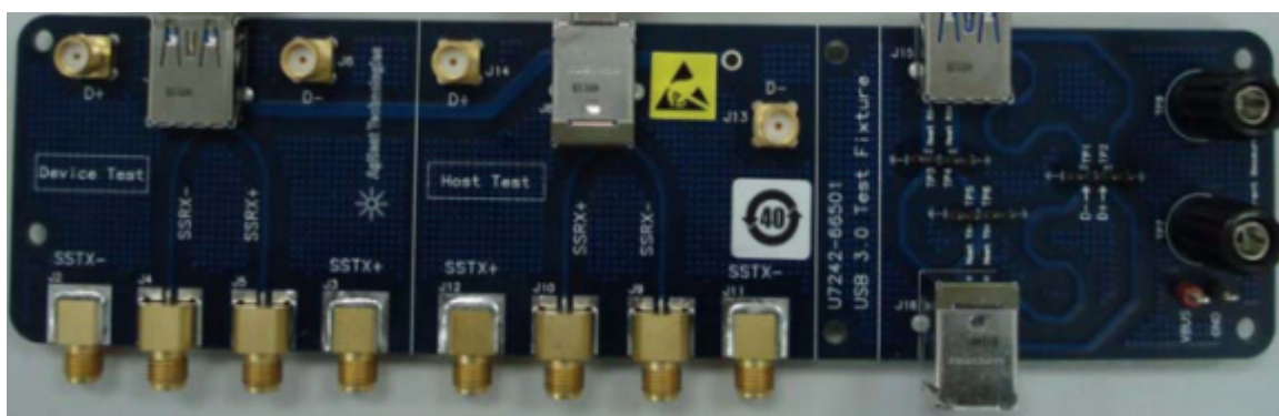
图3-8 Agilent USB 3.0 Tx测试夹具U7242
