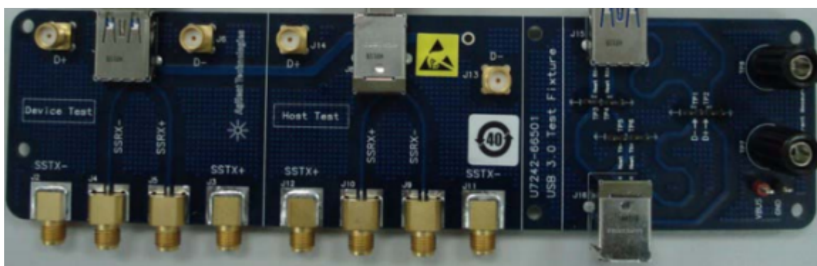
图3-8 Agilent USB 3.0 Tx测试夹具U7242
