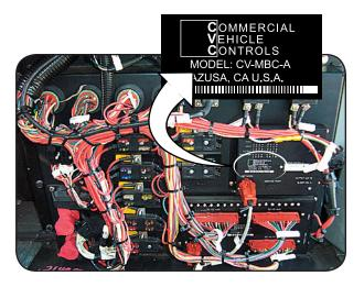
Drill a 5/32 hole to attach the Diode Block connector of the new harness to the PDU box in the location shown. Attach with a short #10 self tapping sheet metal screw. Insert the Diode Block (0081525) into the connector.
