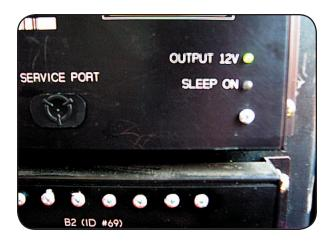
11.4 When the system indicates Sleep Mode, check the current draw. Draw should be between 80 –100 mA, depending upon optional equipment installed.
