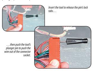
Use the black pin removal tool to remove the wires at the following six locations. Replace each removed wire with the corresponding wire of the new harness:
