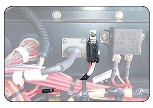
5 Unplug MBC Power connector (far right side of image). Slide yellow pin removal tool over the pin of the green wire (labeled SYS WAKE). Pull the green wire from the connector.
