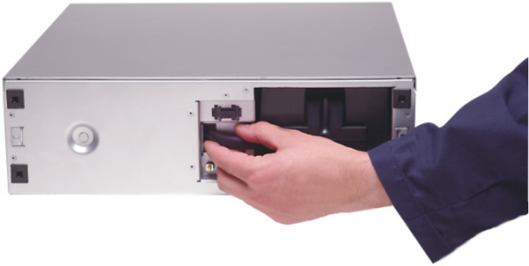
Figure 5. Battery Wire Connection
