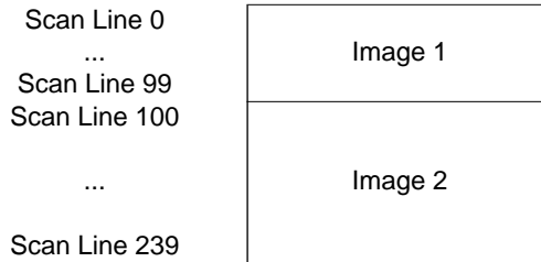
Screen 1 Display Line Count Register = 99 lines
