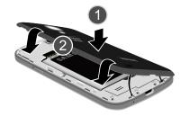
2. Press down along the edge of the back cover (3) until you have a secure seal.
