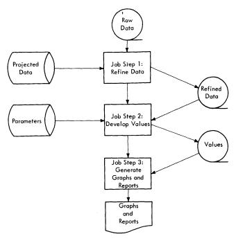
Figure A-3. Input Flow for Example 2
