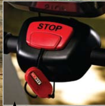
Dual emergency stop for added safety
