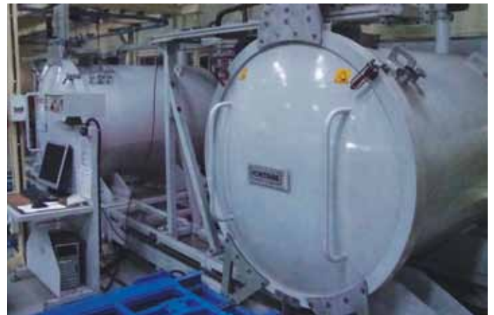
Automatic gas filling and leakage testing station
