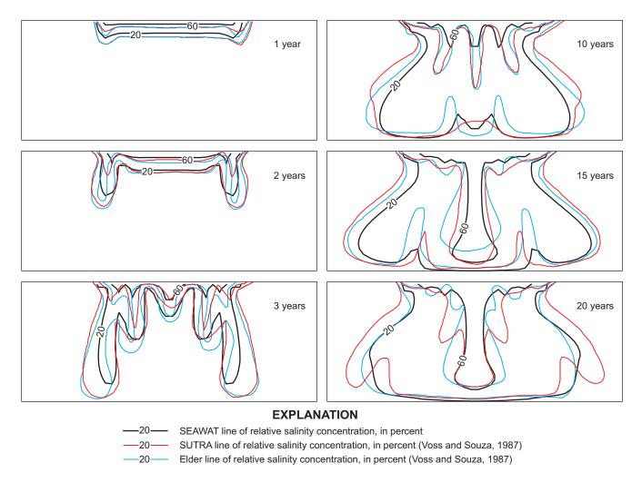
Figure 16. Comparison between SEAWAT, SUTRA, and Elder's solution for the Elder problem over time.
