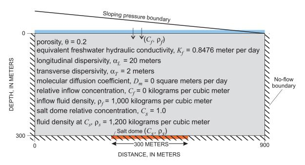
Figure 17. Boundary conditions and model parameters for the HYDROCOIN problem.
