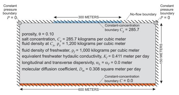
Figure 14. Boundary conditions and model parameters for the Elder problem.
