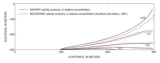
Figure 18. Comparison between SEAWAT and MOCDENSE for the HYDROCOIN problem.
