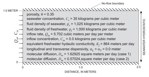
Figure 12. Boundary conditions and model parameters for the Henry problem.
