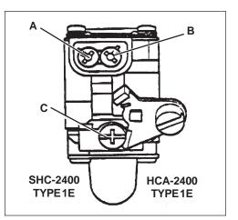
Check idle speed and reset if necessary. If a tachometer is available, idle speed should be set to the specification found on page 12 "Specifications" of this manual.
