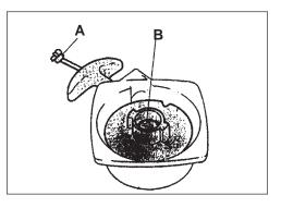
4. Remove the old starter rope and prepare the new rope by first heating both ends to prevent fraying.
