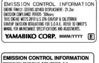
EMISSION CONTROL INFORMATION ENGINE FAMILY: CEHXS.0214KL DISPLACEMENT: 21.2cc EMISSION COMPLIANCE PERIOD: 300Hours THIS ENGINE MEETS 2012 U.S. EPA EXIVEY & CALIFORNIA EXIL EVE EMISSION REGULATIONS FOR S.O.R.E. REFER TO OWNER'S MANUAL FOR MAINTENANCE SPECIFICATIONS AND ADJUSTMENTS. YAMABIKO CORP. MIMM/YYYYY
