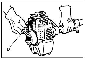
starts and runs. Release throttle trigger and allow unit to warm up at idle for several minutes.
