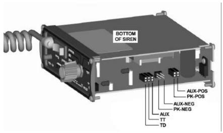
**Auxiliary Input Polarity** - The auxiliary input (green wire) is normally activated by applying a positive voltage to the wire. To activate by connecting to ground (negative), move the jumper from the "AUX-POS" pins to the "AUX-NEG" pins.
