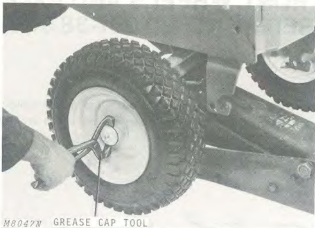
Fig. 3-Removing Front Wheel Components from Axle
