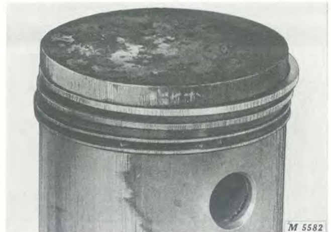
Fig. 16-Scratched Ring Faces Caused by Abrasives in the Engine
