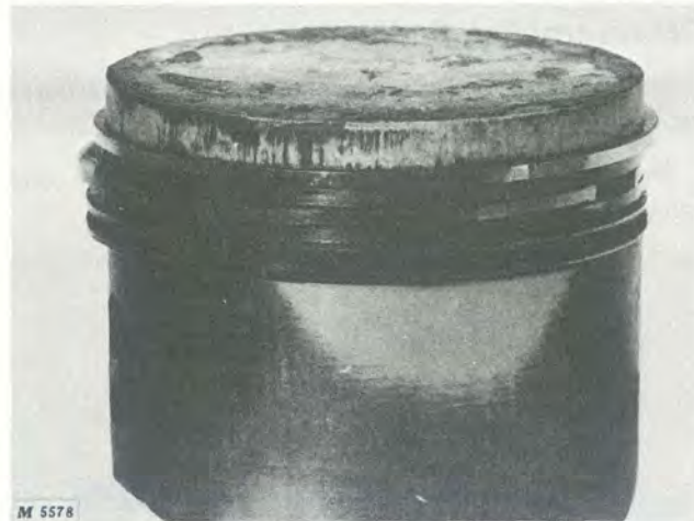
Fig. 12-Scored Piston and Rings Caused by Overheating as Temperatures Reach Melting Point of the Materials
