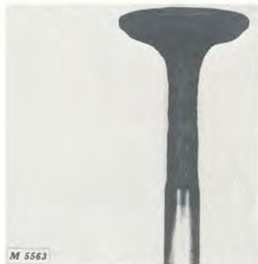
Fig. 3 - Valve Stem Corrosion
