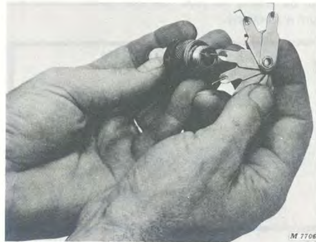
Fig. 11-Checking Spark Plug Gap
