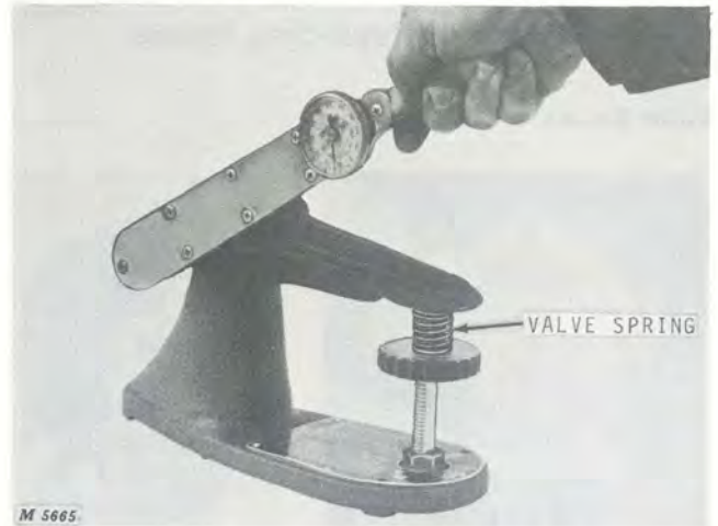
Fig. 11 - Valve Spring Tension
