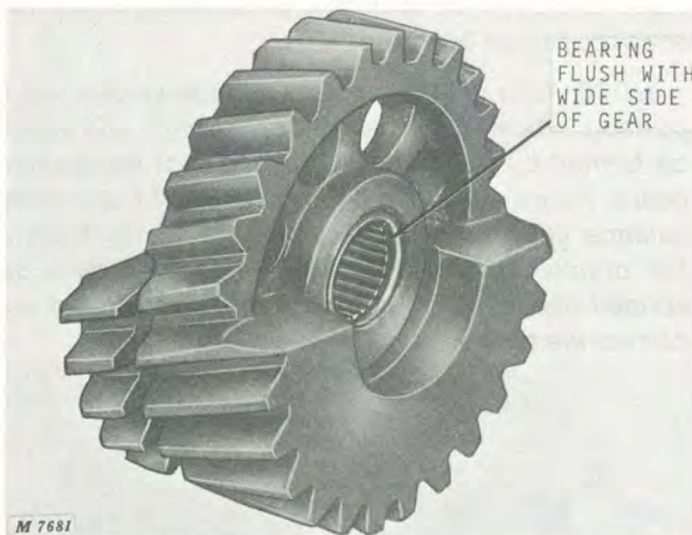
Fig. 36-Installing Needle Bearing in Gear
