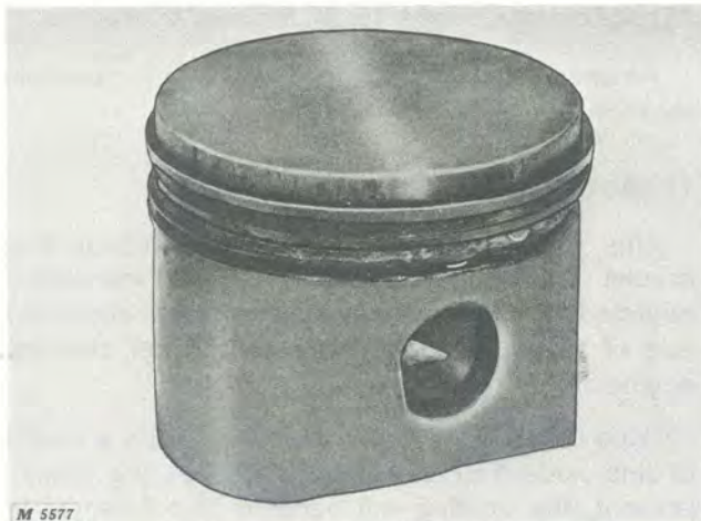
Fig. 25-Piston Damage Caused by Piston Pin Retainer Coming Loose
