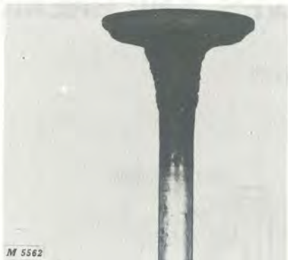
Fig. 2 - Lead Deposits on Leaky Intake Valve
