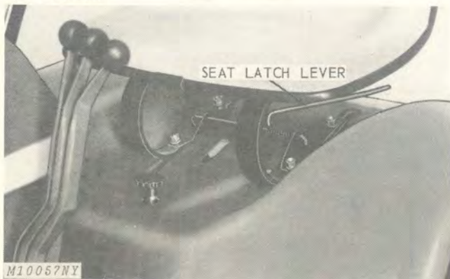
Fig. 8-Seat Adjusting Components (Serial No. 38,001-46,500)
