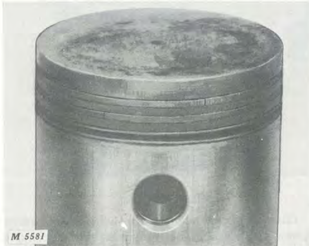
Fig. 15-Piston Rings Stuck and Broken Because of Lacquer, Varnish and Carbon Build-up
