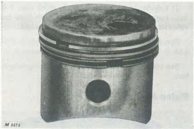
Fig. 23-Hole Burned in Piston Caused by Pre-Ignition
