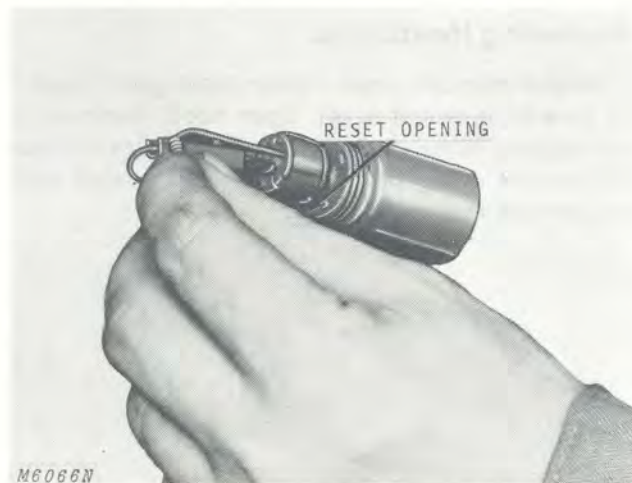
Fig. 10-Resetting Circuit Breaker in Cigarette Lighter
