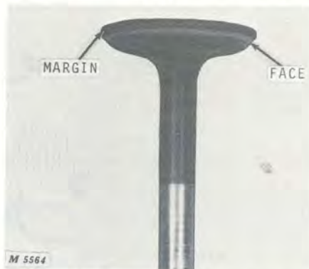
Fig. 4 - Exhaust Valve Running Too Hot
