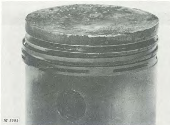
Fig. 17-Worn Oil Rings Which Cannot Provide Oil Control
