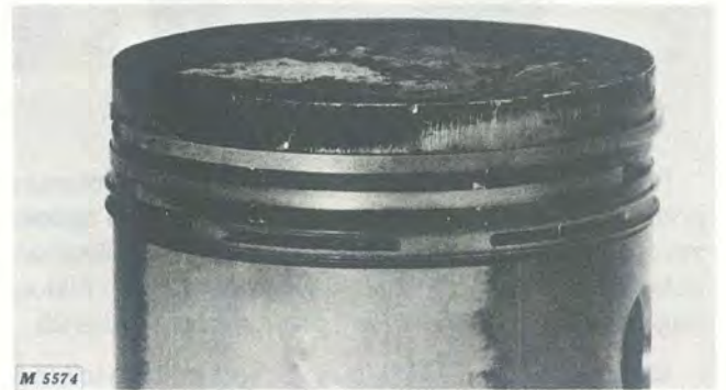
Fig. 22-Piston Top Land Burning Caused by Detonation
