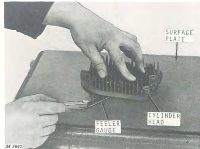
Fig. 9 - Checking Surface of Cylinder Head
