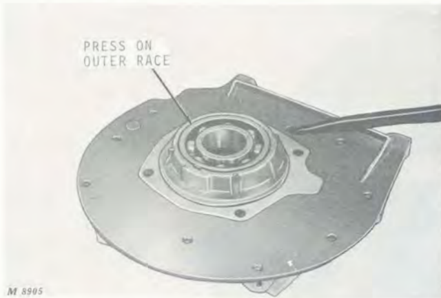
Fig. 43-Installing Main Bearing in Bearing Plate
