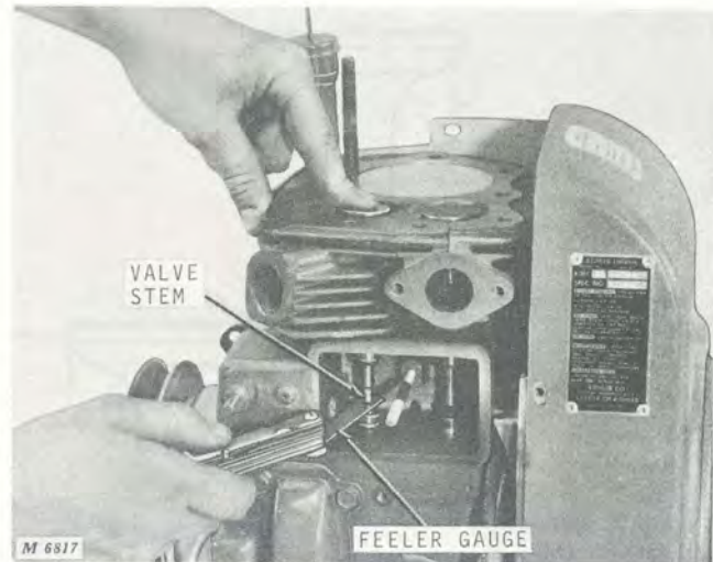
Fig. 21 - Checking Valve Clearance
