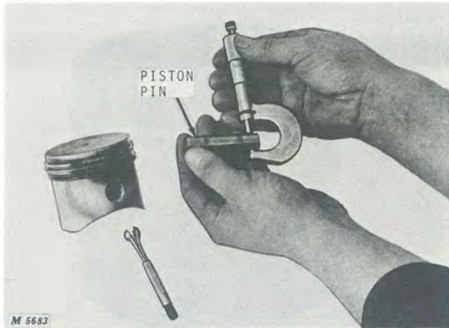
Fig. 20-Measuring Piston Pin and Piston
