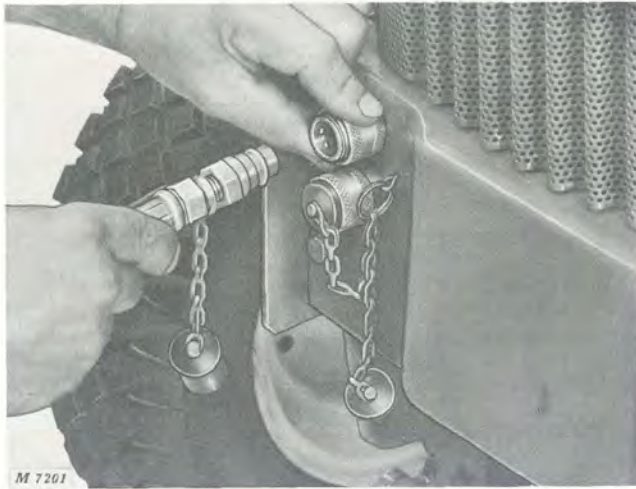
Fig. 3-Connecting Hose to Front Coupler
