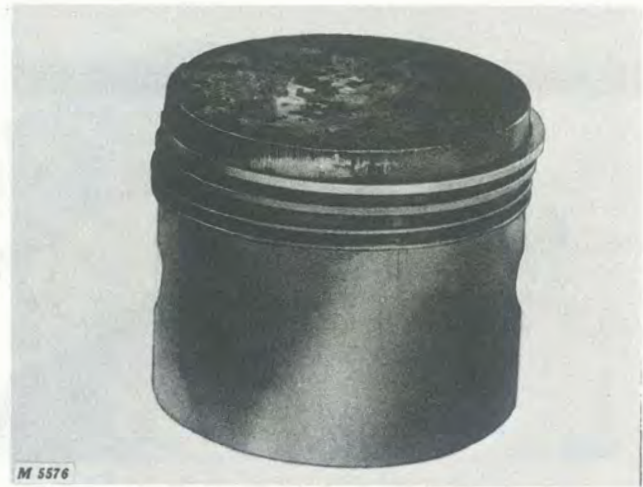
Fig. 24-Diagonal Piston Wear Pattern Caused by Bent or Twisted Connecting Rod
