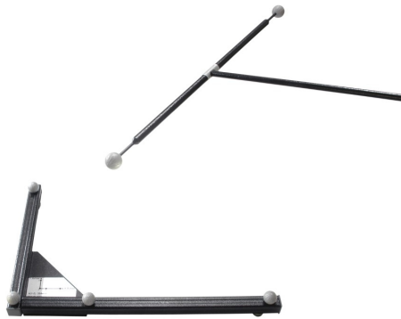
Figure 4.33: A room calibration set consisting of angle and wand
