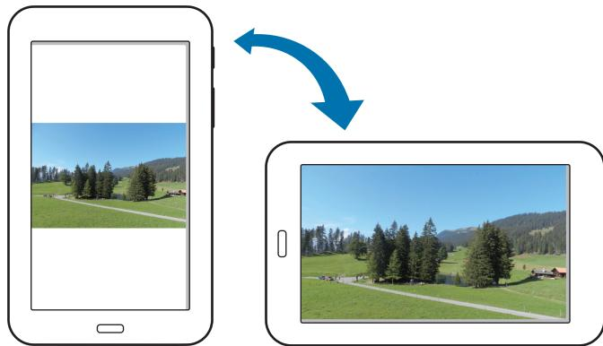
To prevent the display from rotating automatically, open the notifications panel and deselect **Screen rotation**.
