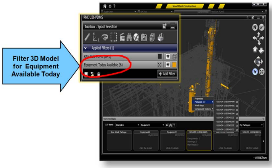
Figure 2: Filters in SmartPlant Construction enable users to find material and equipment availability.
