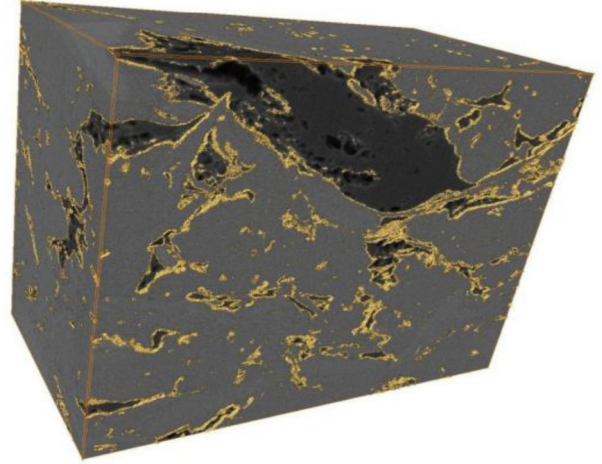
Figure 2—3D SEM segmentation showing kerogen network, yellow outlines the kerogen network (Ambrose et al. 2010).
