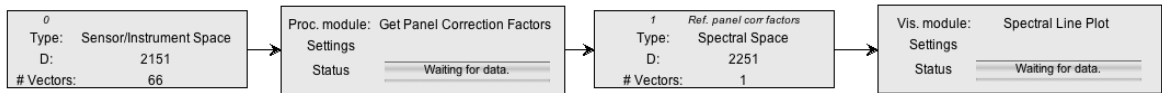
Figure 83: Processing chain selecting the correction factors and plotting them as a Spectrum.
