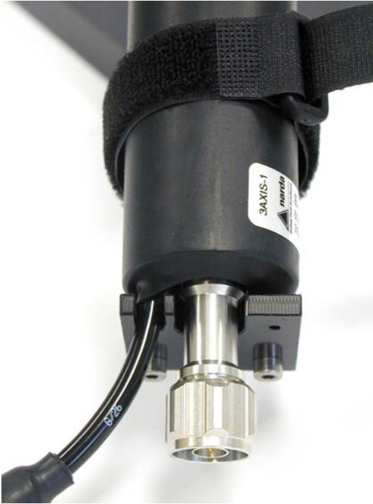
Figure 6: Cable and N connector in guideway
