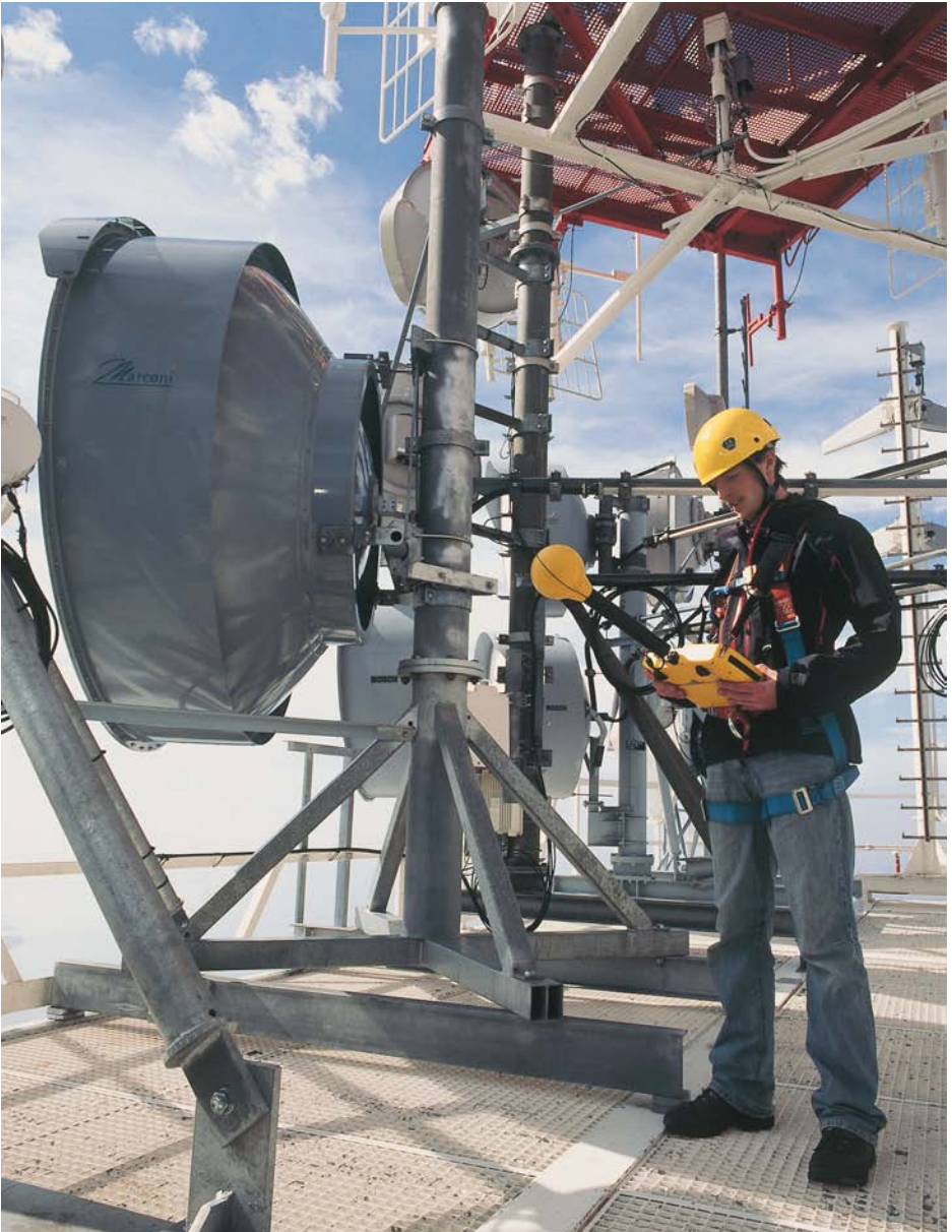
Figure 1: SRM-3006 in on-site use
