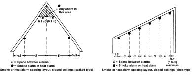
Alarms shall first be spaced and located within 3 ft. (0.9m) of the peak or high side of the ceiling, measured horizontally. The number and spacing of additional alarms, if any, shall be based on the horizontal projection of the ceiling.
