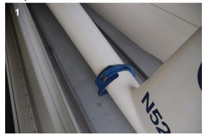
Using a lifting strap, lift the tail boom and walk it aft until fuselage dolly is at end of ramp
