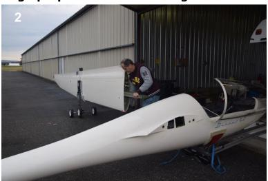
Ease wing into position, keeping pins aligned, refine wing dolly height if needed
