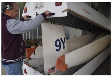
Pull safety clips and latch pins, open latches at aft end of trailer
