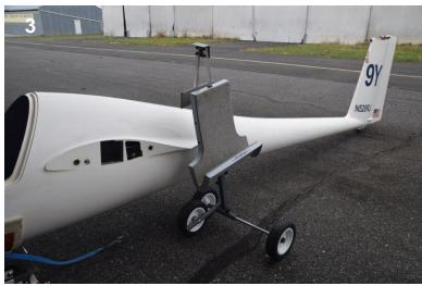
Unfasten and remove the tie-down strap that runs through the spar opening
