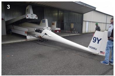
Roll the tail out until the tail wheel is at the aft stop of the ramp, monitor boom clearance
