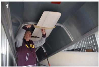
Slide tail onto aft pins, pull rigging tool to open forward fitting, seat and close, remove tool
