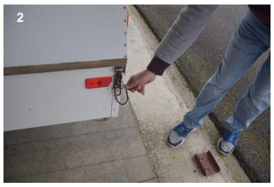
Release the sliding latch pin from the left side of the aft lower door
