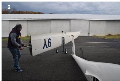
With main spar pin fully seated, secure with safety clip
