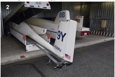
Open canopy, check cockpit condition, locate spar pin, rigging tool, winglets, checklist
