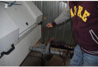
Pull out the sliding ramp, check alignment, unfold the center rail
