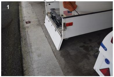
When aft door is straight down and firmly set, trailer is stabilized and ready to unload
