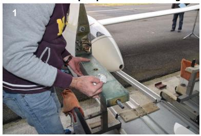
Safety clip for the main spar pin is stowed on the parachute static line ring, left aft cockpit
