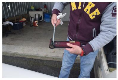
Position wing stand 2/3 of the way out the wing, then lower and remove wing dolly
