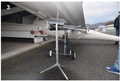
Insert spar pin only one inch into left wing spar, rotate handle to left side wall
