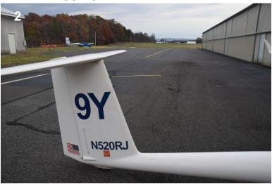
Install tail dolly, check tire pressures, move glider from trailer area, secure trailer
