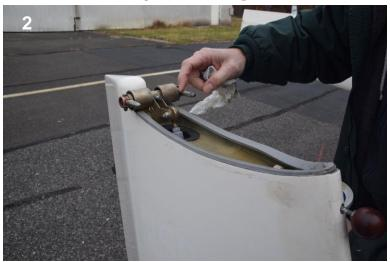
Remove stock wing tips, align winglet spar pin, push in to seat
