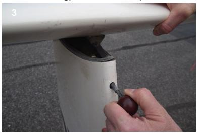
Clean and lubricate elevator bayonet pins and forward attach point fittings
