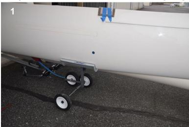
Rotate wing to level, rest end of spar in hole, clean & lube 7 pins and receivers
