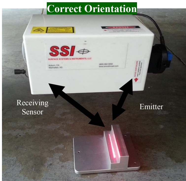
Figure 36: The Block Orientation for the Height Verification Test
