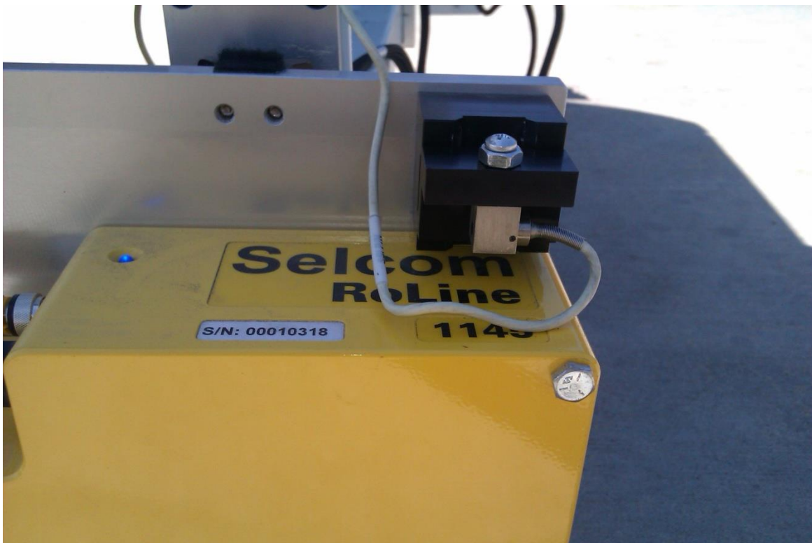
Figure 18: The accelerometer upside down
