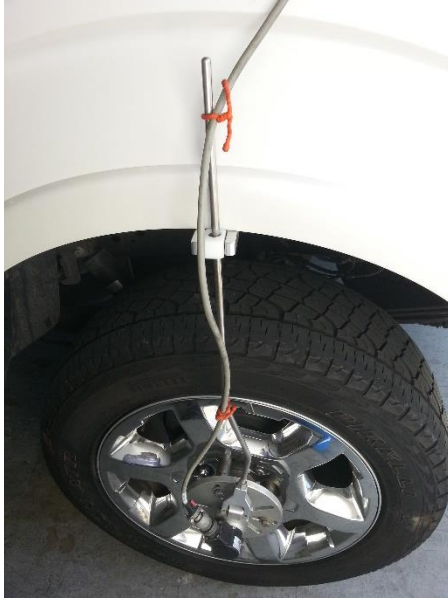
Figure 7: The DMI pole and receiver
