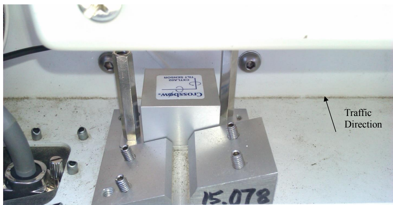
Figure 22: The inclinometer on the flat plate for a rear-mount.
