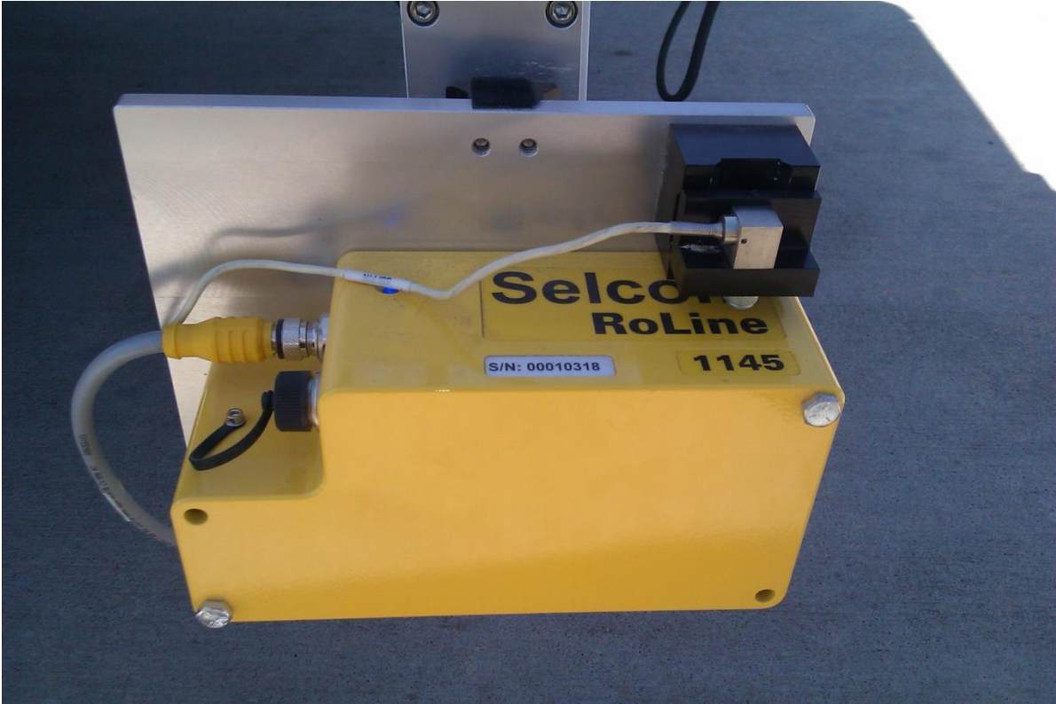
Figure 17: The upright accelerometer position
