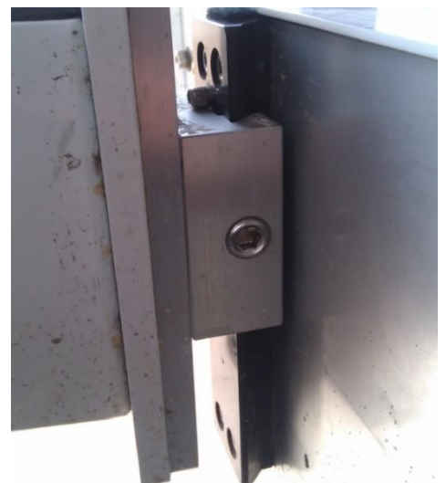
Figure 11: The vertical dovetail and laser plate assembly
