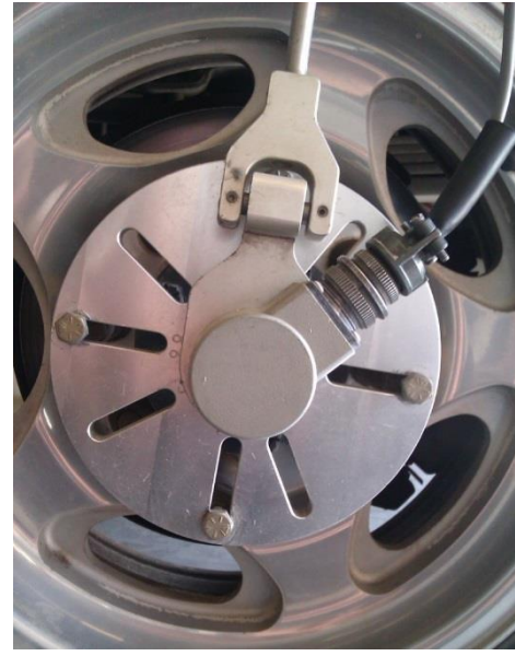
Figure 8: The DMI wheel attached to an 8-lug vehicle with a 4-lug extender configuration.
