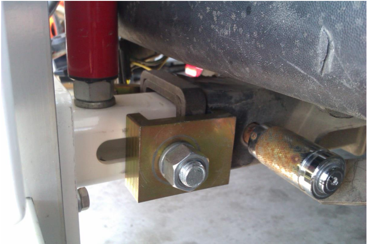
Figure 9: The hitch receiver mount with lock brackets.
