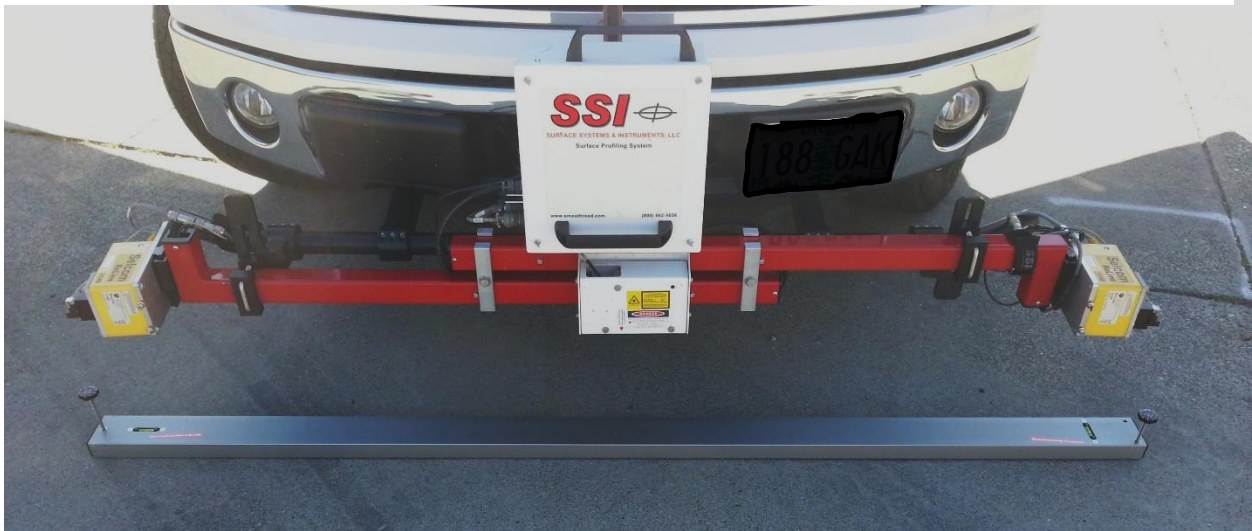
Figure 24: A three laser system with a level straightedge for inclinometer
