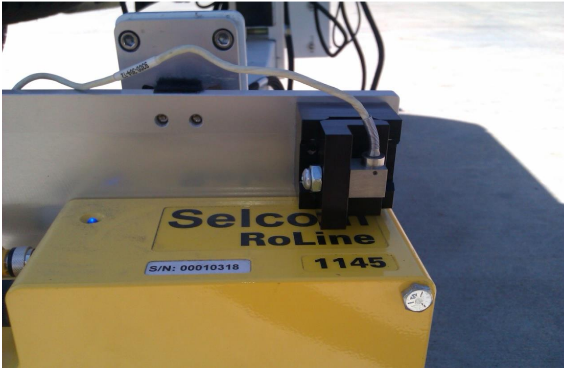
Figure 19: The accelerometer on its side
