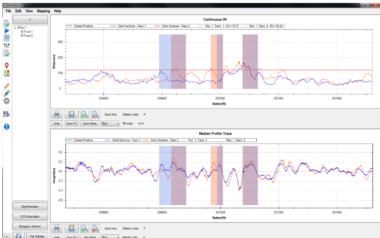
Figure 119: Grinding Navigation with green current location displayed
