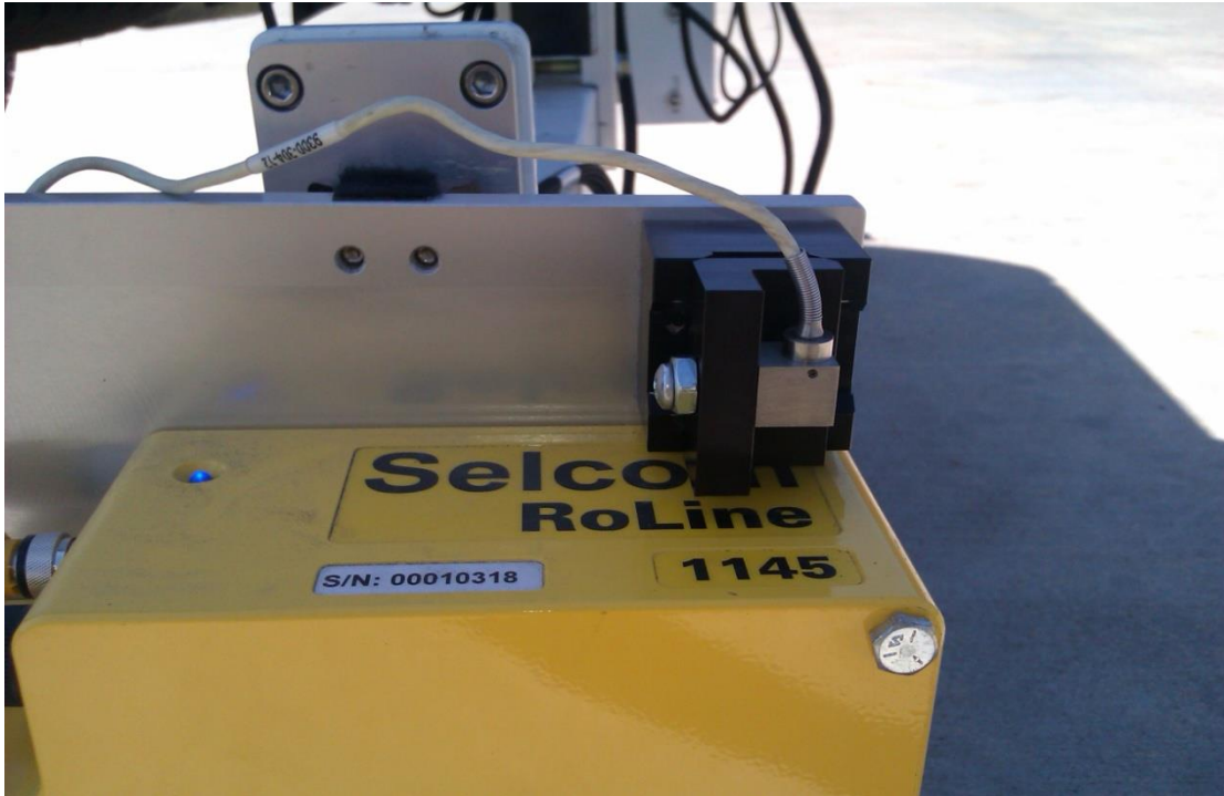
Figure 19: The accelerometer on its side
