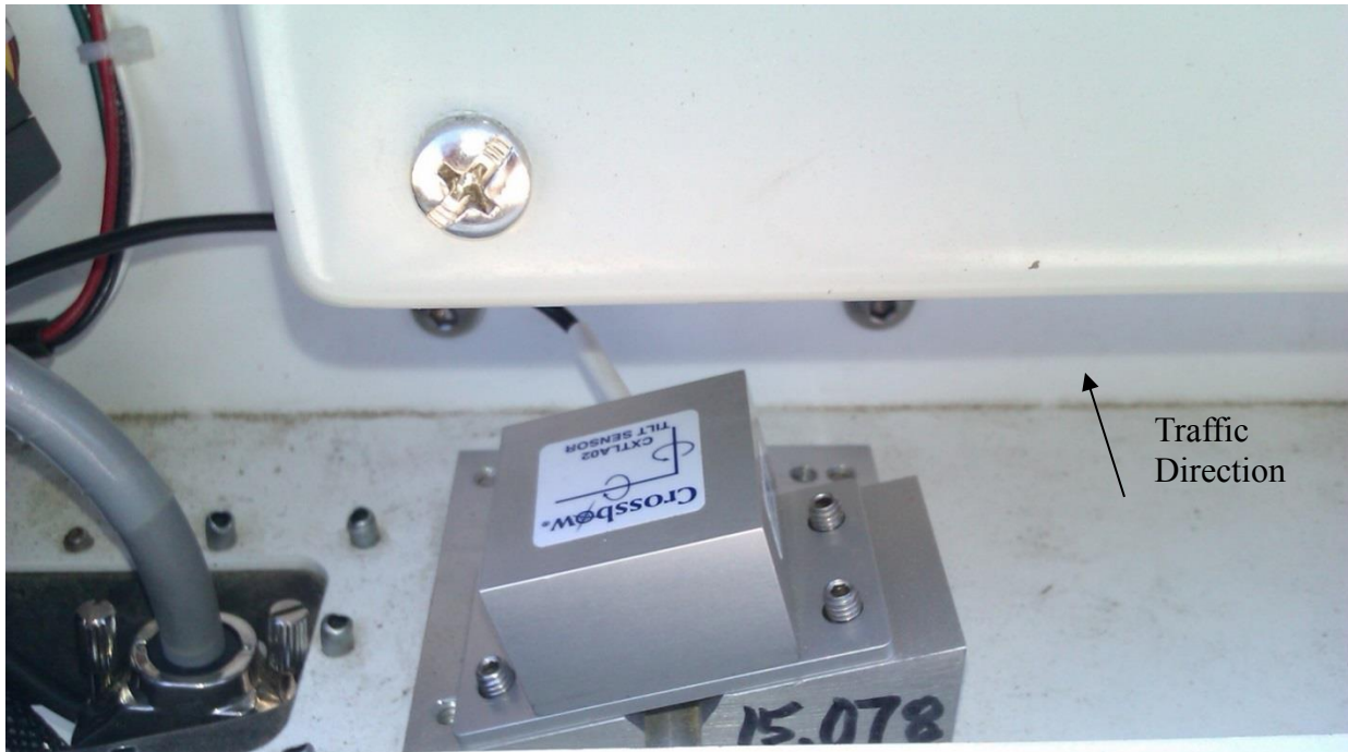
Figure 23: The inclinometer on the angled plate for a rear-mounted system
