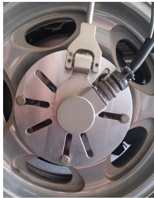
Figure 7: The DMI wheel attached to an 8-lug vehicle with a 4-lug extender configuration.
