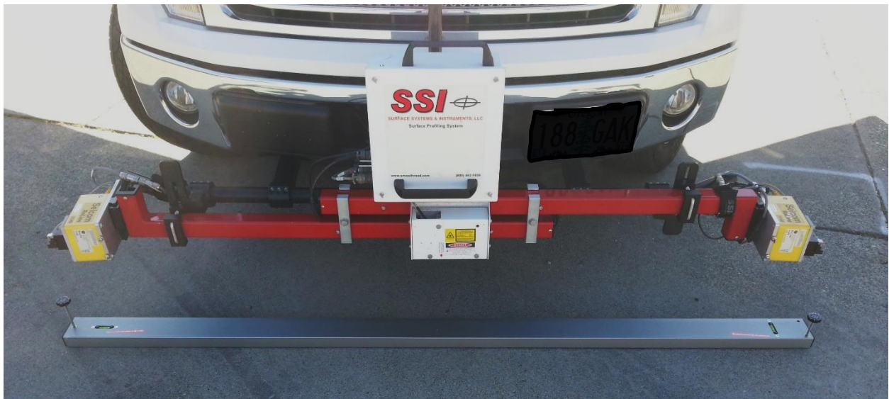
Figure 24: A three laser system with a level straightedge for inclinometer
