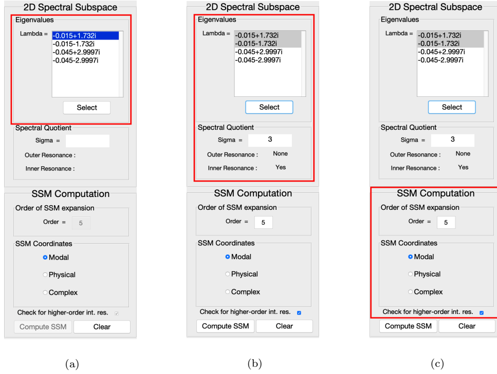
Fig. 2.4: (a) Analyzing the spectrum of the linearized system at the trivial fixed point. (b) Selecting a two-dimensional spectral subspace \mathcal{E} . (c) Specifying the order of the Taylor expansions and choosing the desired output coordinates.
