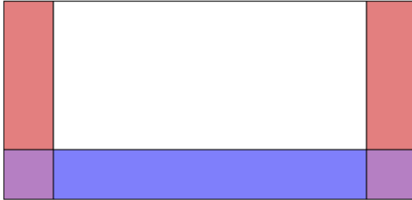
Figure 3.3: A vertical cross-section through the computational domain with a free surface boundary along the top edge. The original seismic wave equation is solved the white region. The wave speed is reduced in the normal direction of the surrounding super-grid layers, where also a high order damping term is added.
