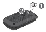
Use the groove at the top left corner of the cover (3) to lift the cover up and away from the back of the phone (4).
