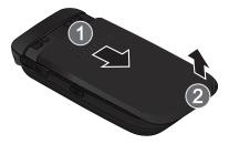
Insert the battery (label side up as shown) into the battery compartment so that the metal contacts on the phone match up with those on the battery.
