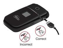
Plug the flat end of the charger into the phone's power/accessory interface connector and the other end into an electrical outlet.
