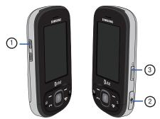
Volume keys: allows you to adjust the ringer volume while in standby mode or adjust the voice volume during a call. When receiving an incoming call, briefly press down either
