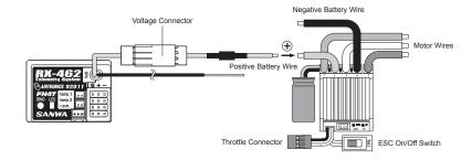
If the voltage connector is not connected to the positive terminal of your ESC, plug the voltage connector into an empty channel slot in your receiver. If the receiver cannot detect voltage an alarm will continuously sound.
