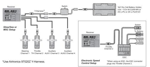
Do NOT use servos rated for 4.8 or 6.0 volts with a 2S Li-Po or 2S Li-Fe/A123 receiver battery pack or damage to the servos could result
