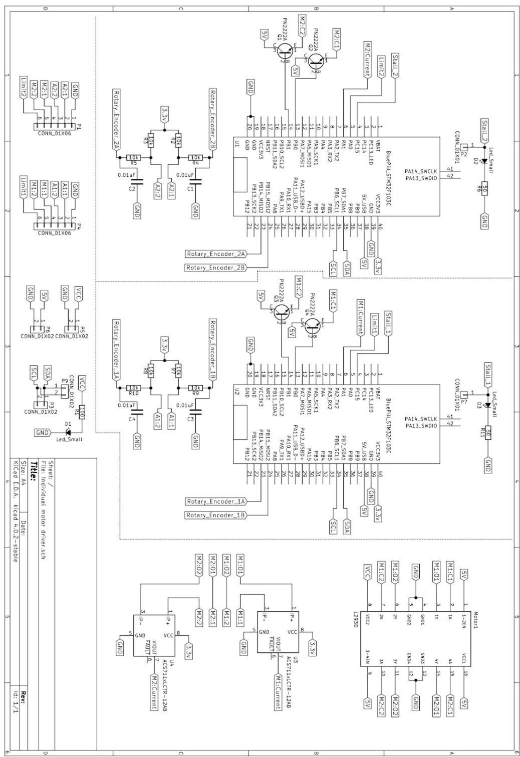
**C. PC Communication Board:** The PC communication board is another STM32 “Blue Pill” board that is used as the “master” controller. Using a USB to TTL converter board a computer can connect to the to the arm through USB. The communication board then uses I2C to communicate with all of the controller microcontrollers and to coordinate the movement of the arm. It does not have its own power supply and is only powered when plugged into a computer.
