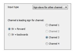
First of all, it has to be specified which direction is indicated by the 5 V value. A voltage value of 0 V automatically indicates the opposite direction.
