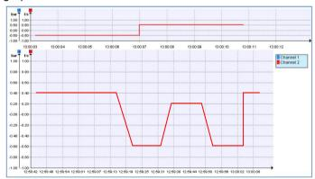
The continuous curves in the top diagram show the last 10 taken values. The bottom diagram shows the entire realtime measurement:
