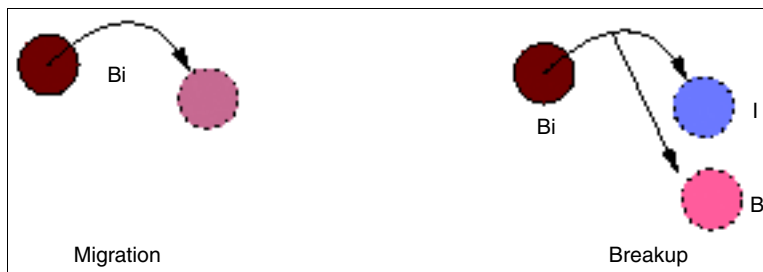
Figure 45 Impurity pairs can diffuse or break up into a substitutional plus an interstitial or a vacancy
