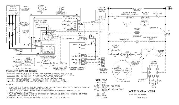
Figure 10: Wiring Diagram
