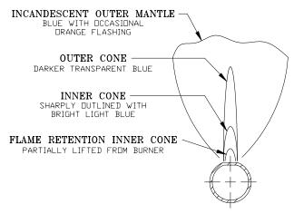
Figure 16: Main Burner Flame
