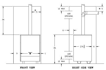
\* MINIMUM RADIAL CLEARANCE ARDUND VENT PIPE
