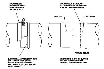
Figure 8: Typical Joint Detail
