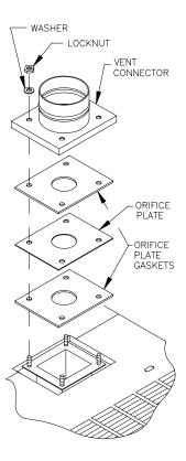
Figure 7: Vent Connector Installation
