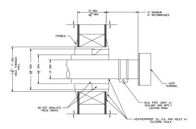
Figure 9: Recommendations for Thimble and Wall Penetration
