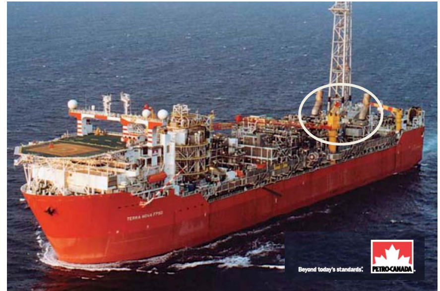
Terra Nova FPSO, Two GE Frame 6B
