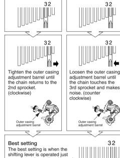
enough to take up the play and the chain touches the 3rd sprocket and makes noise.
