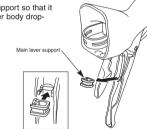
Replacing the cable guide Use this hole to replace the cable guide.
