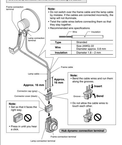
Secure the cable to the front fork or the basket stay so that it will not get caught in the spokes or any other parts while riding. If the position of the hub dynamo may change with respect to the lamp while riding, for example when using a suspension fork, make sure that the cable is connected so that it will not be too loose or too tight at any point within the range of movement.
