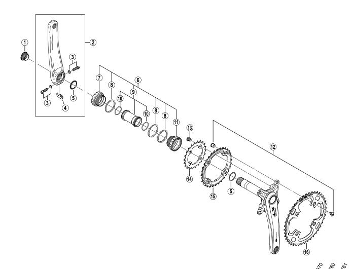
Bolt circle diameter: 104 mm...(For outer gear and middle gear), 64 mm...(For inner gear)
