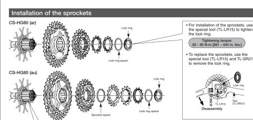
For each sprocket, the surface that has the group mark should face outward and be positioned so that the wider part of each sprocket and the A part (where the groove width (0) is wide) of the freewheel body are aligned.
