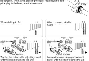
barrel until the chain touches the 3rd sprocket and makes noise. (counter clockwise)
